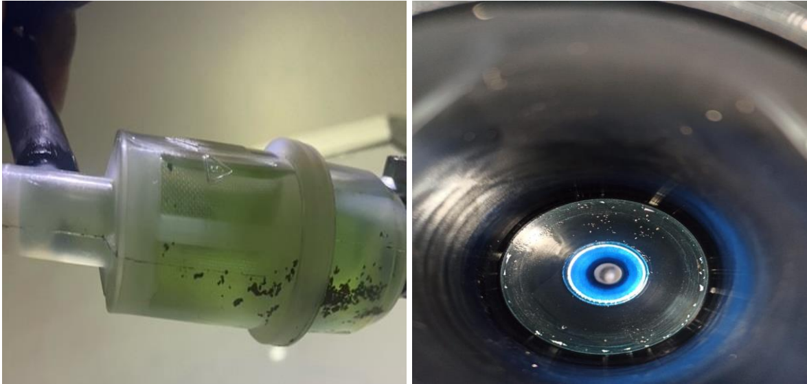
Figures 6 and 7: Metal particles inside the left tank fuel filter (left picture). Foreign particles found inside the fine fuel filter (right picture).
