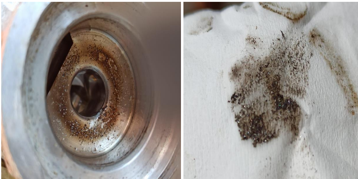
Figures 8 and 9: Dirt found inside the fuel pressure regulator (left picture). The cloth used to clean the fuel pressure regulator (right picture).
