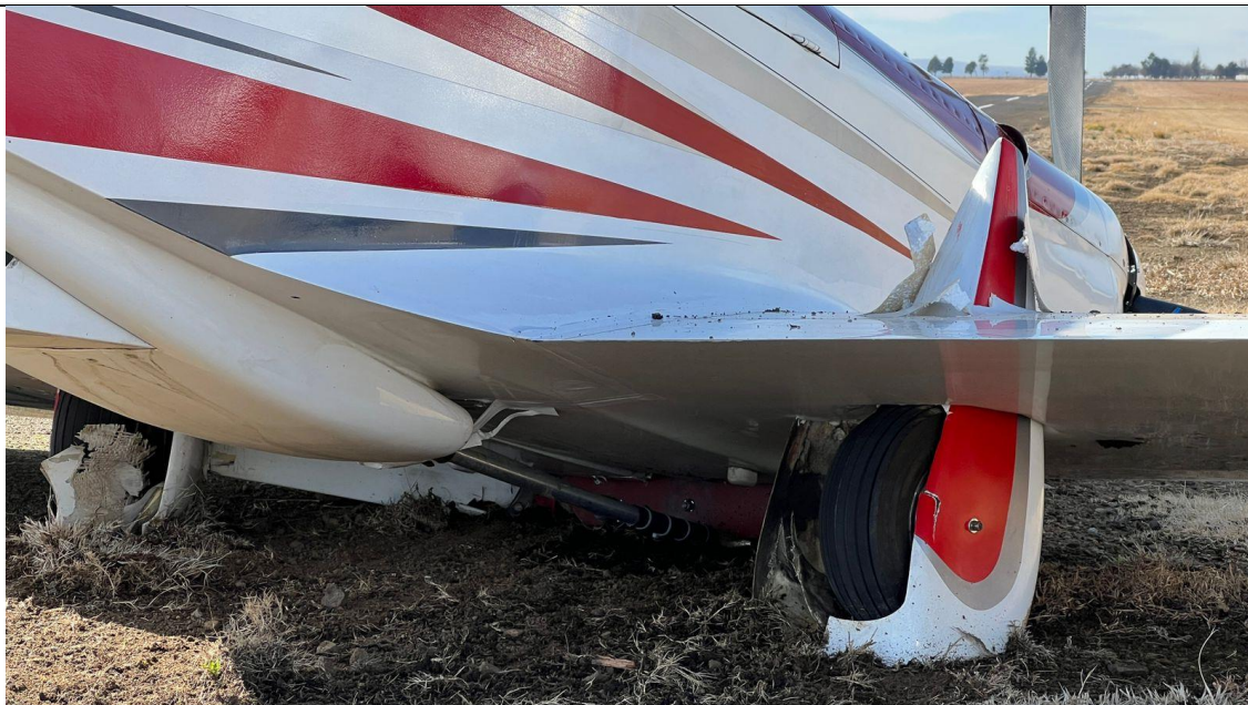
Figure 4: Landing gear penetrated the wings on both sides. (Source: Disaster Management)
