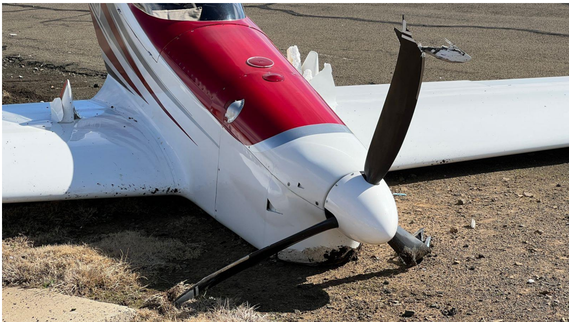
Figure 3: Damage to the propeller. (Source: Disaster Management)
