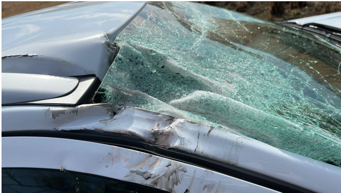
Figure 7: Impact markings from the aircraft on the vehicle. (Source: Disaster Management)
