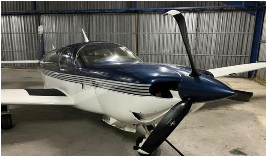
Figure 3: The bent propeller blades. (Source: Operator)
