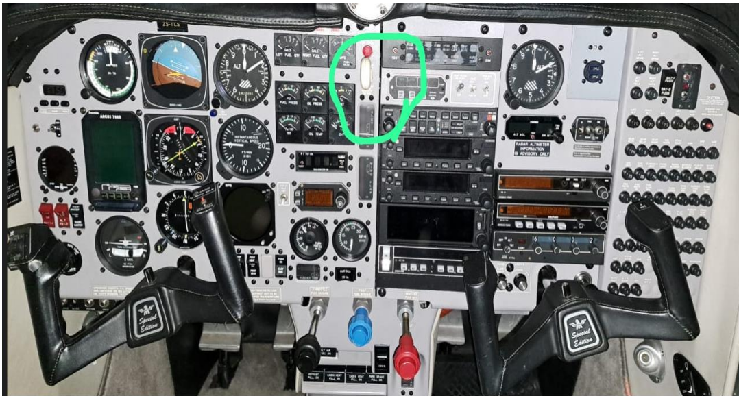
Figure 1: The instrument panel showing the landing gear control lever in the UP position.
