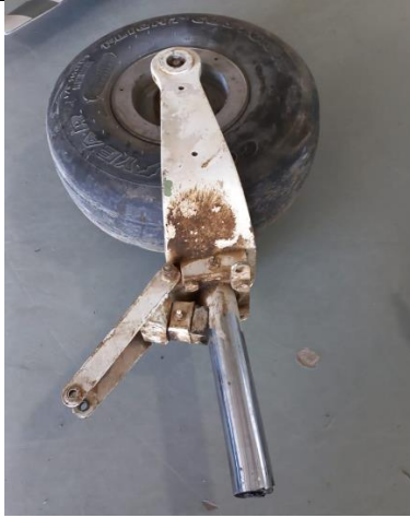
Figures 3 and 4: The separated nose gear wheel (left), and the severed oleo and torque link (right) (Source: Operator)
