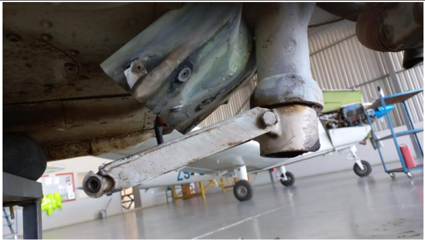
Figures 3 and 4: The separated nose gear wheel (left), and the severed oleo and torque link (right) (Source: Operator)
