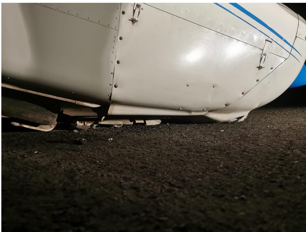
Figure 2: The collapsed nose landing gear. (Operator)
