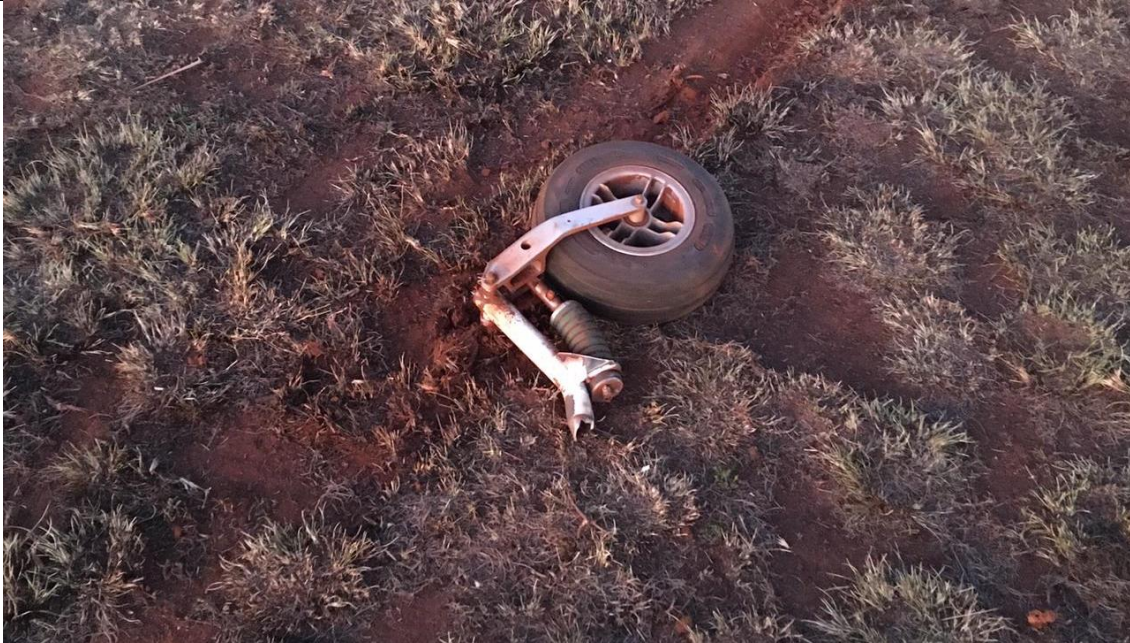
Figure 3: The detached nose gear assembly. (Source: Pilot)
