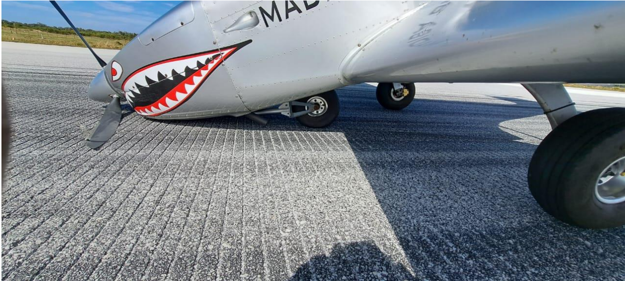
Figure 2: The bent nose gear and the damaged propeller. (Source: Pilot)
