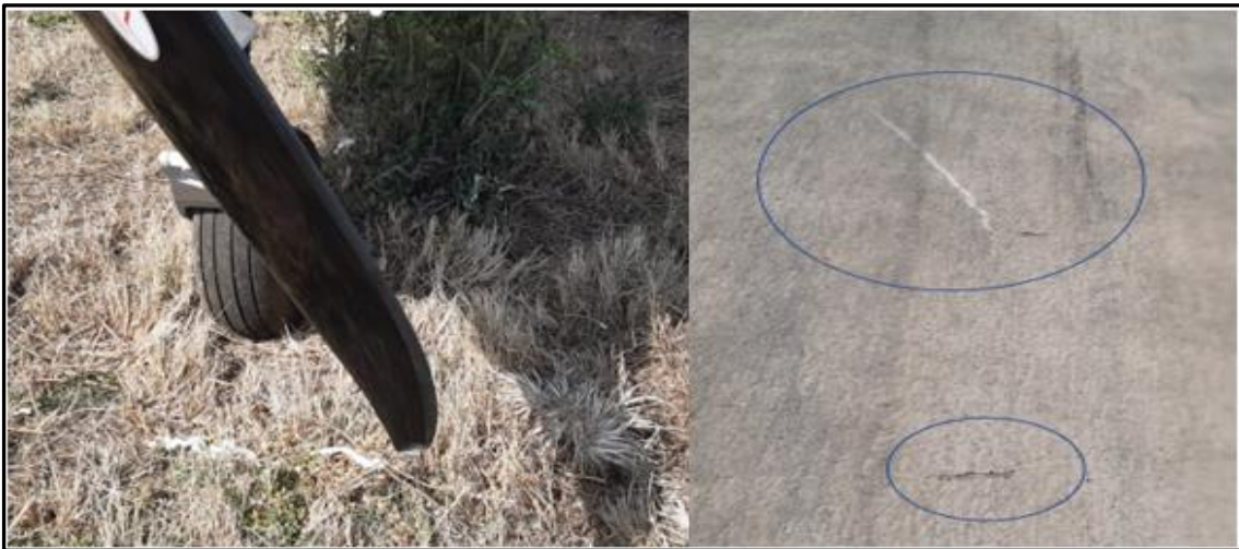
Figure 2: Damage on one of the propeller blades tip (left), and the propeller strike marks on the runway surface (right).
