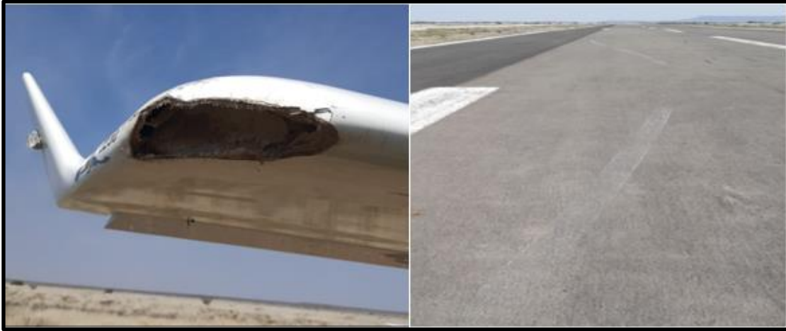
Figure 1: Damage to the right-wing tip (left) and the wing scrape marks on the runway surface (right).
