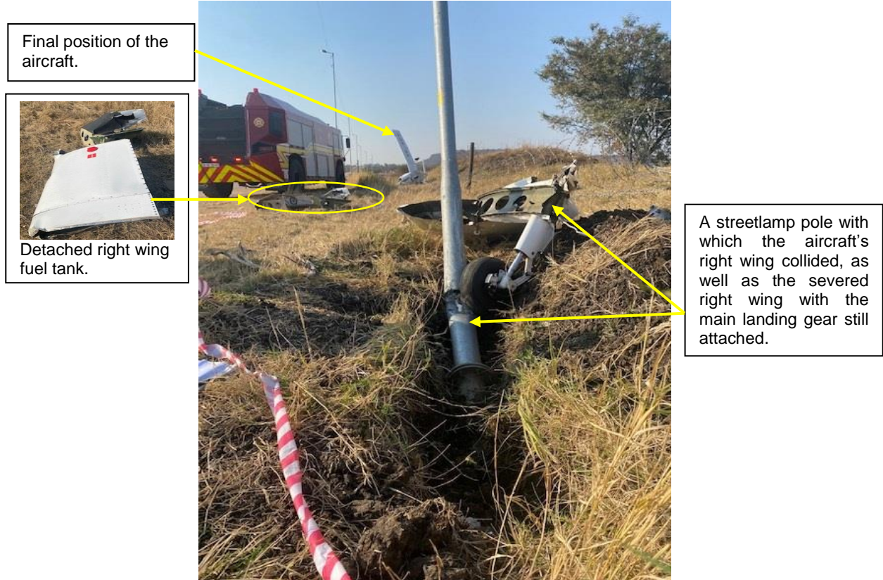
Figure 8: The wreckage layout at the accident site.
