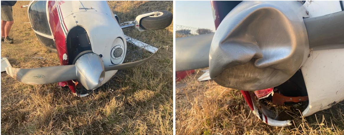
Figures 6 and 7: The propeller as found at the accident site (left picture). The dented spinner (right picture).
