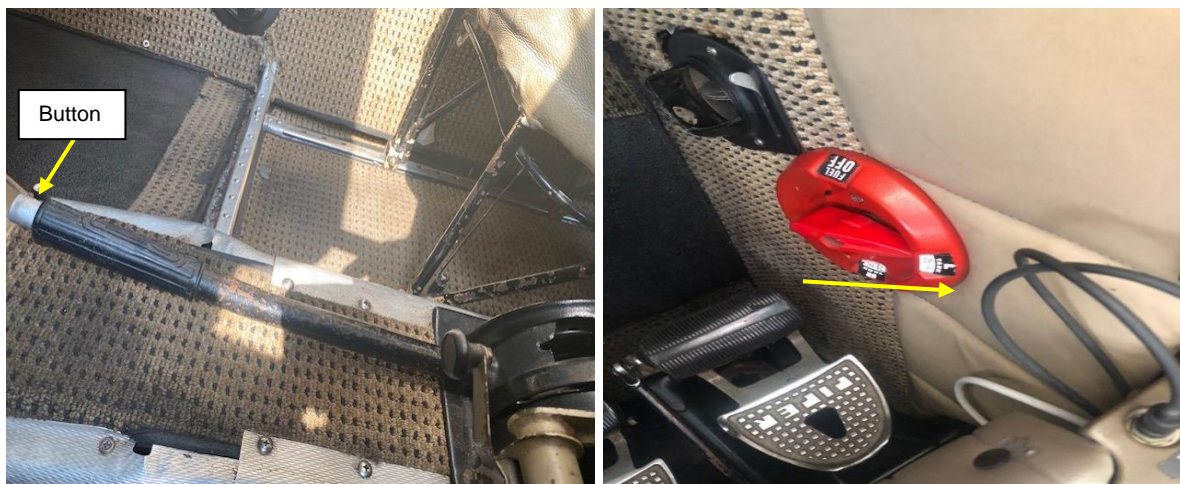
Figures 4 and 5: Flap operating lever in its lowest detent (left picture). The fuel selector valve set to the left tank.
