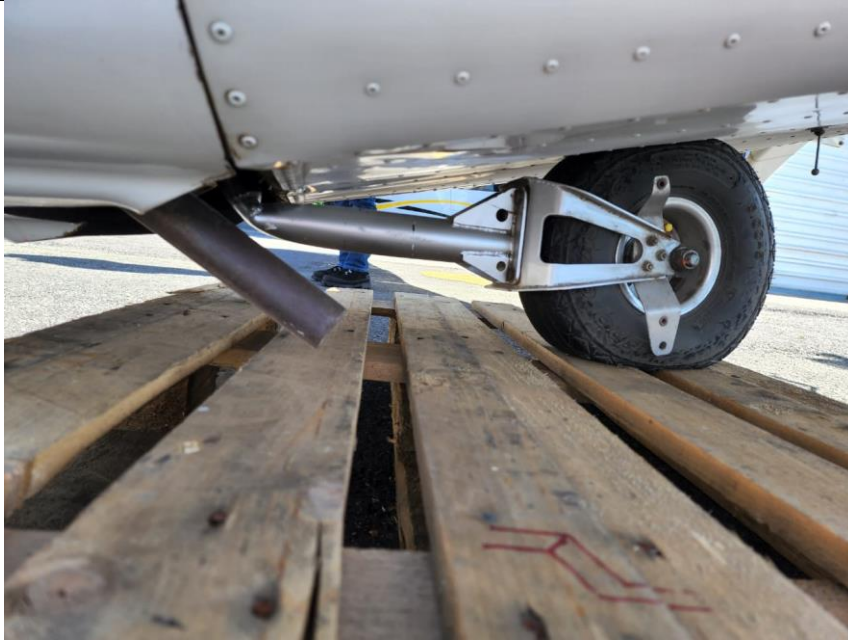
Figure 3: The bent nose gear. (Source: ATO)
