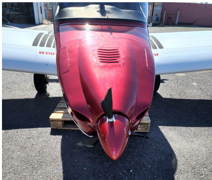
Figure 2: The broken propeller blades. (Source: ATO)
