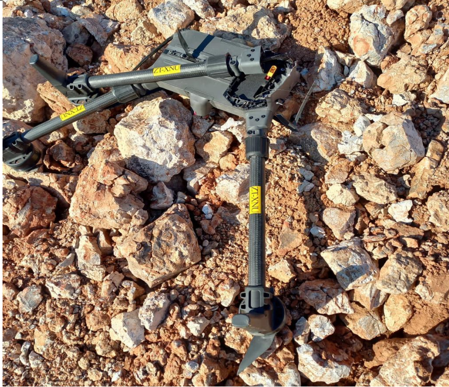
Figure 1: The RPA at the accident site. (Source: Operator)
