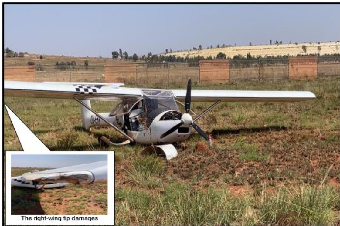
Figure 3: The aircraft at rest. The inset picture shows the damage on the right-wing tip.
