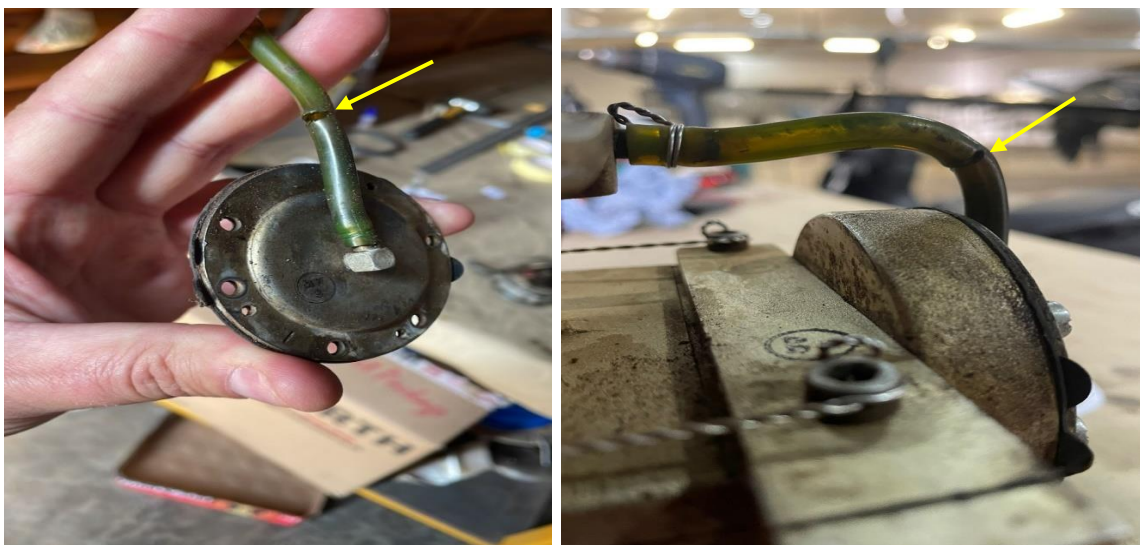
Figures 4 and 5: Pictures of the damaged Tygon plastic air hose/pipe.
