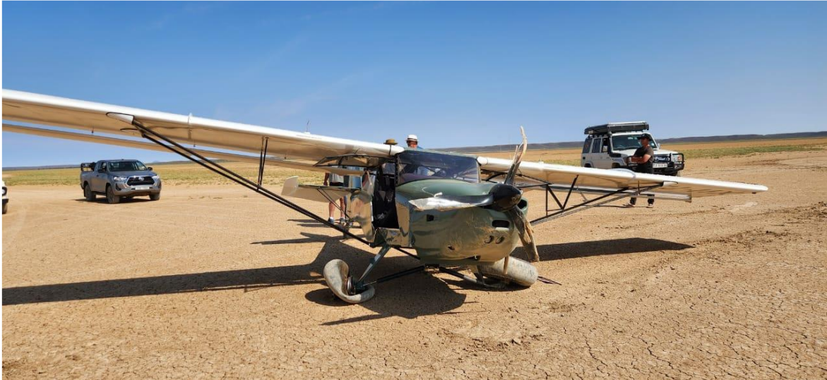
Figure 1: Damaged landing gears and the propeller blades. (Source: Pilot)
