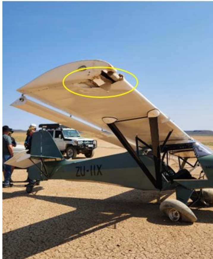
Figure 2: Damaged right-side wingtip. (Source: Pilot)
