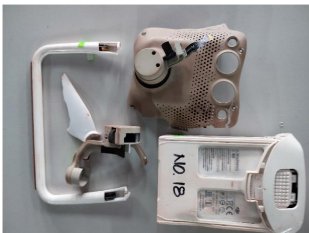
Figures 2 and 3: Damaged battery, propeller blade, gimbal and skid. (Source: Operator)
