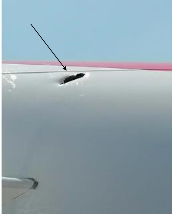
Figure 2: An arrow showing damage to the fuselage. (Source: Operator)
