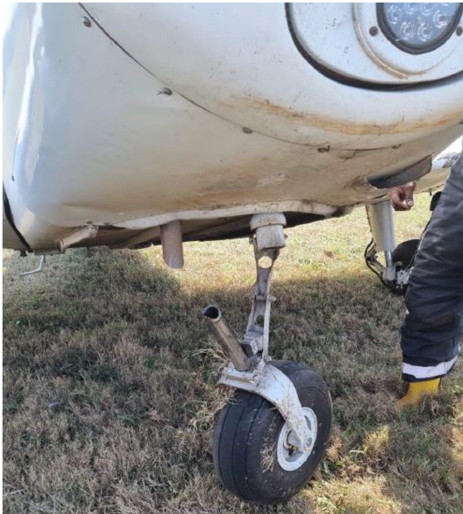
Figure 2: The damaged nose landing gear. (Source: Operator)
