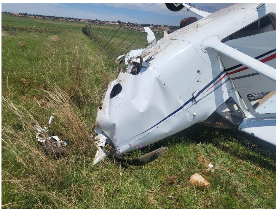
Figure 4: The severed nose undercarriage and bent propeller blades.
