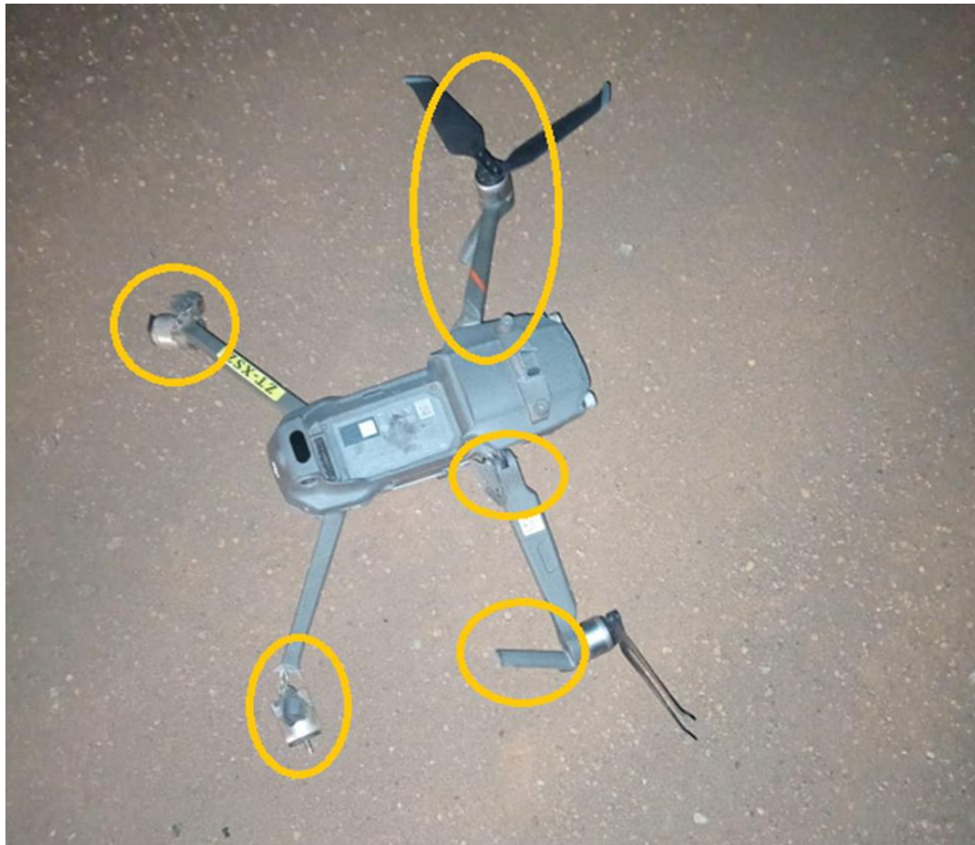
Figure 2: The damage sustained by the ZT-XSZ. (Source: Pilot)
