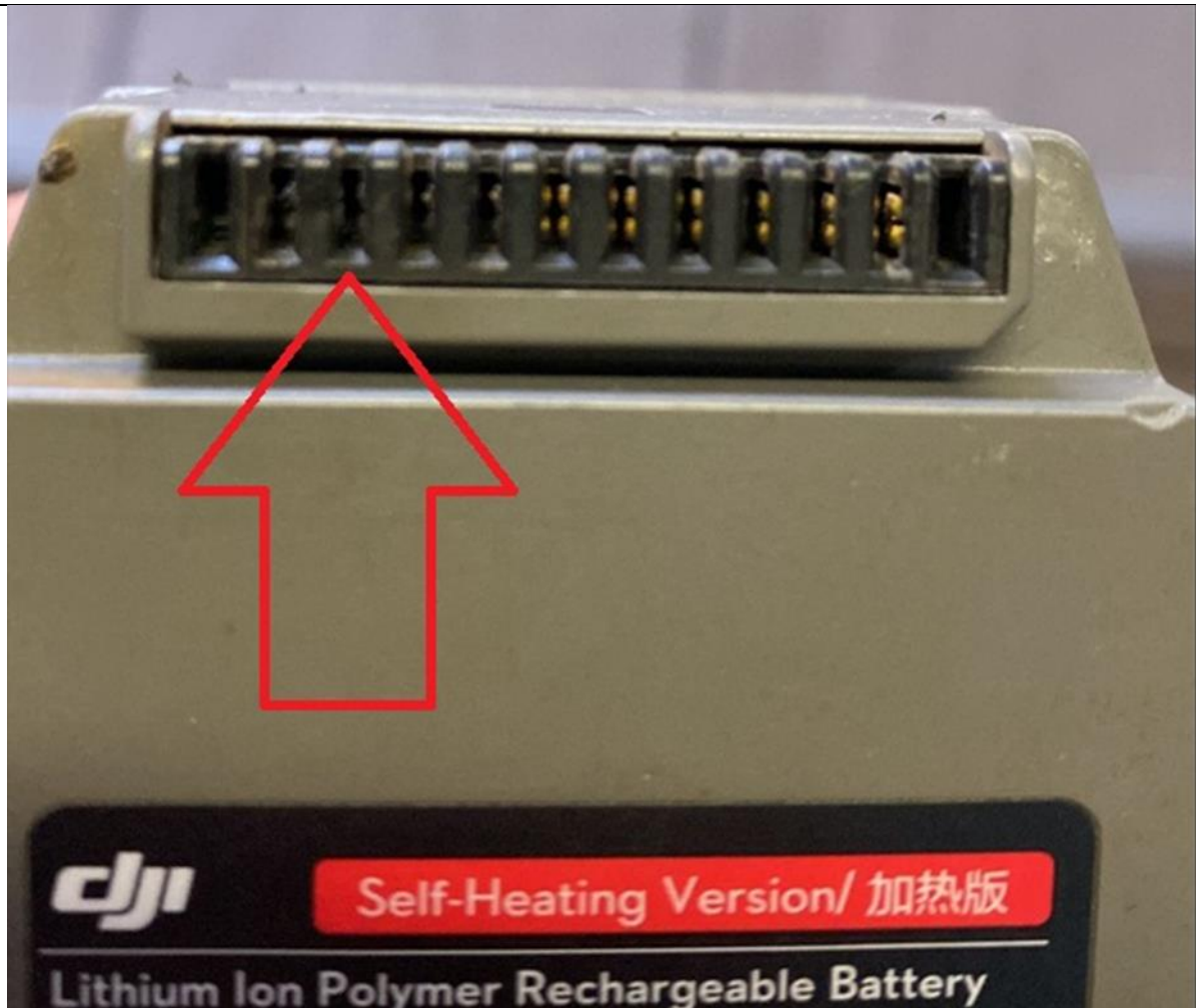
Figure 3: The damaged battery terminals. (Source: Operator)
