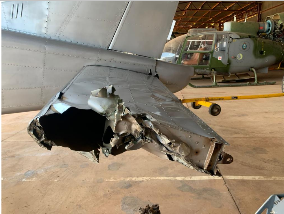
Figure 5: Side view of the damaged left horizontal stabiliser. (Source: Pilot)
