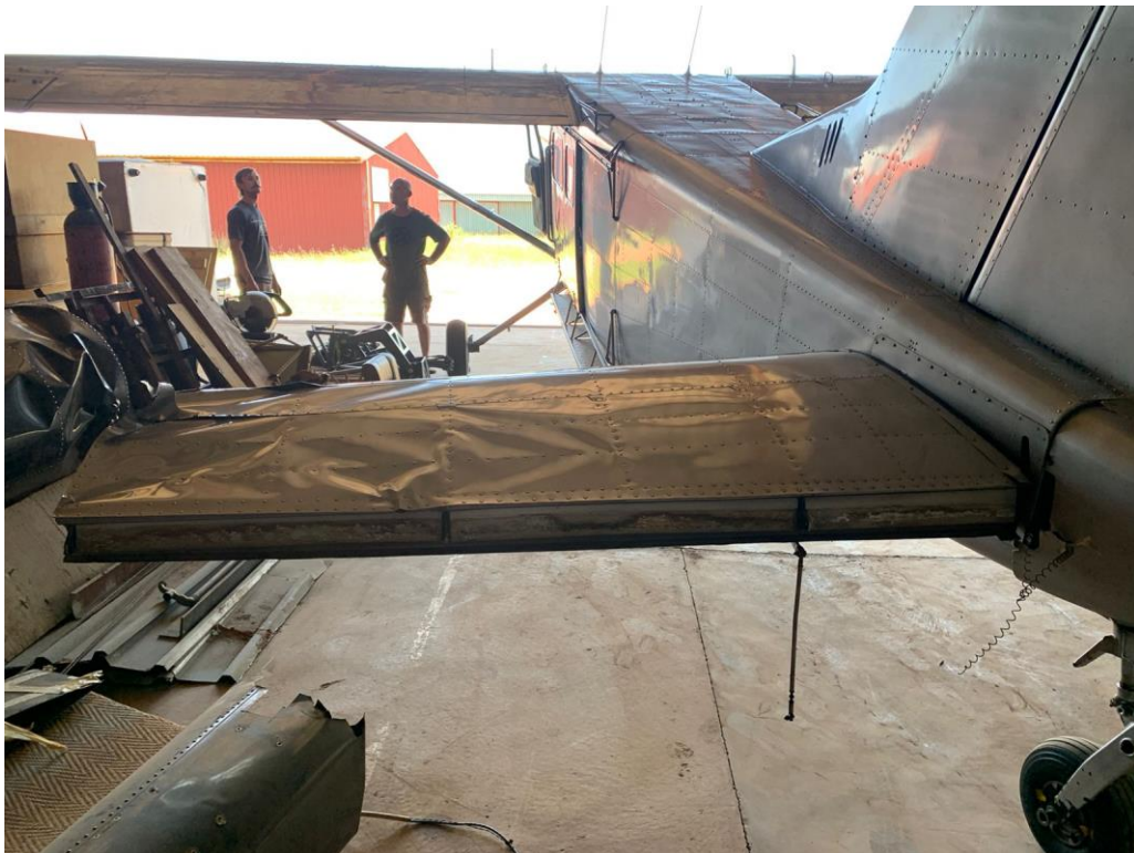
Figure 4: Rearview of the damaged horizontal stabiliser. (Source: Pilot)
