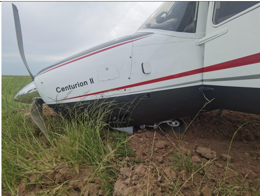
Figure 5: The damaged nose wheel and propeller blades. (Source: Pilot)
