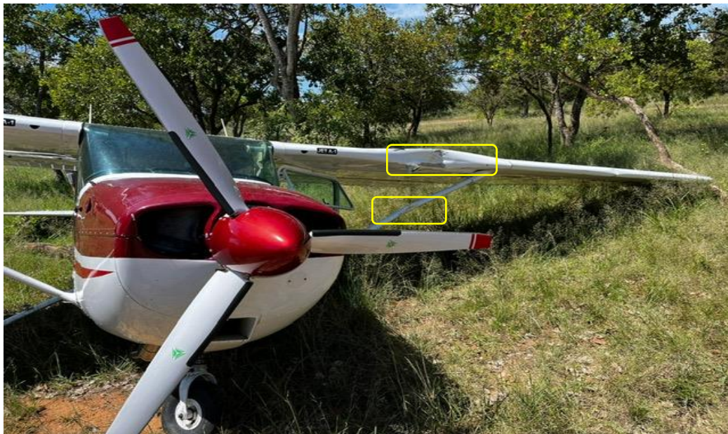
Figure 3: The aircraft at the accident site with sustained damage highlighted in the yellow windows. (Source: Pilot)
