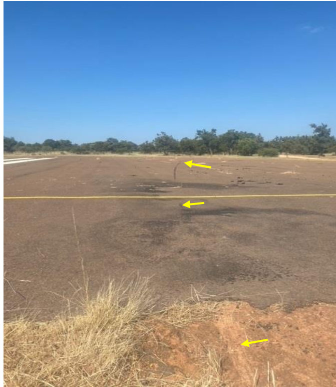
Figure 4: The skid mark made by the right main gear wheel tyre as the aircraft passed the movement before coming to a stop between the trees.
