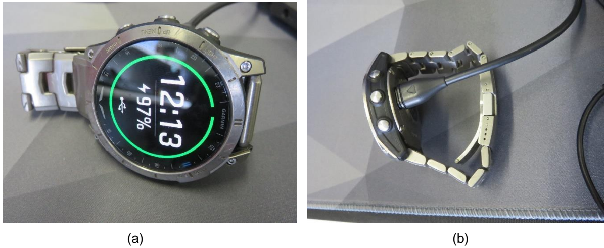
Figure 5: The wristwatch (a), and the download cable attached to it (b).
