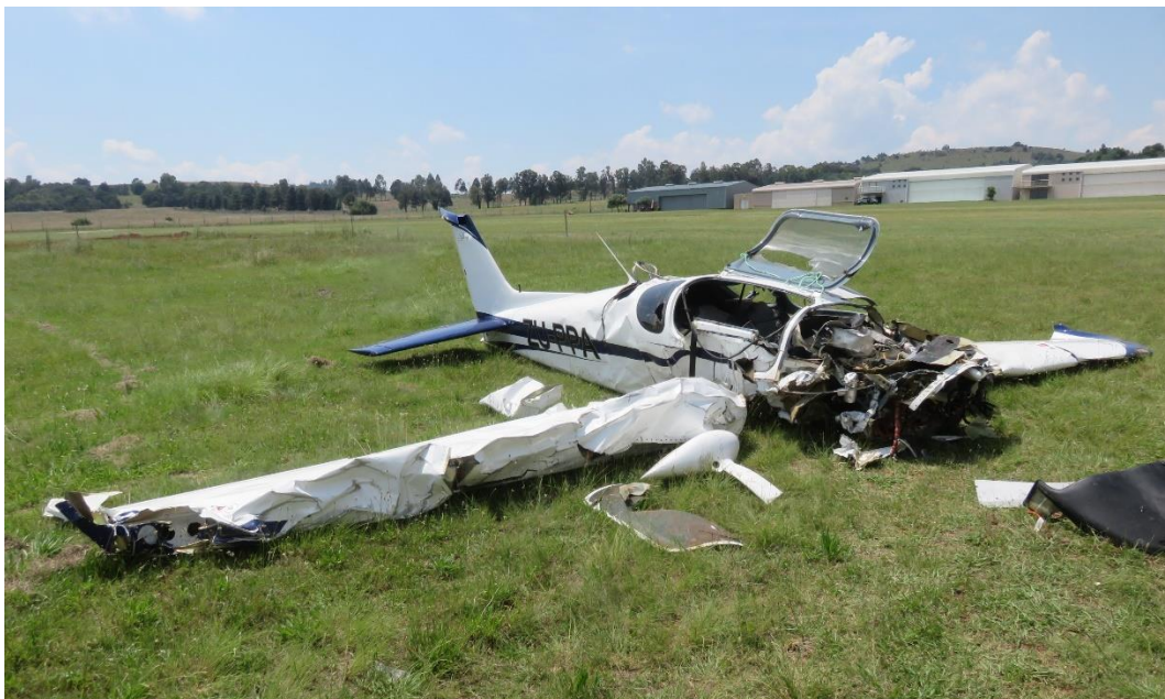
Figure 10: The wreckage layout post-recovery with the engine removed.
