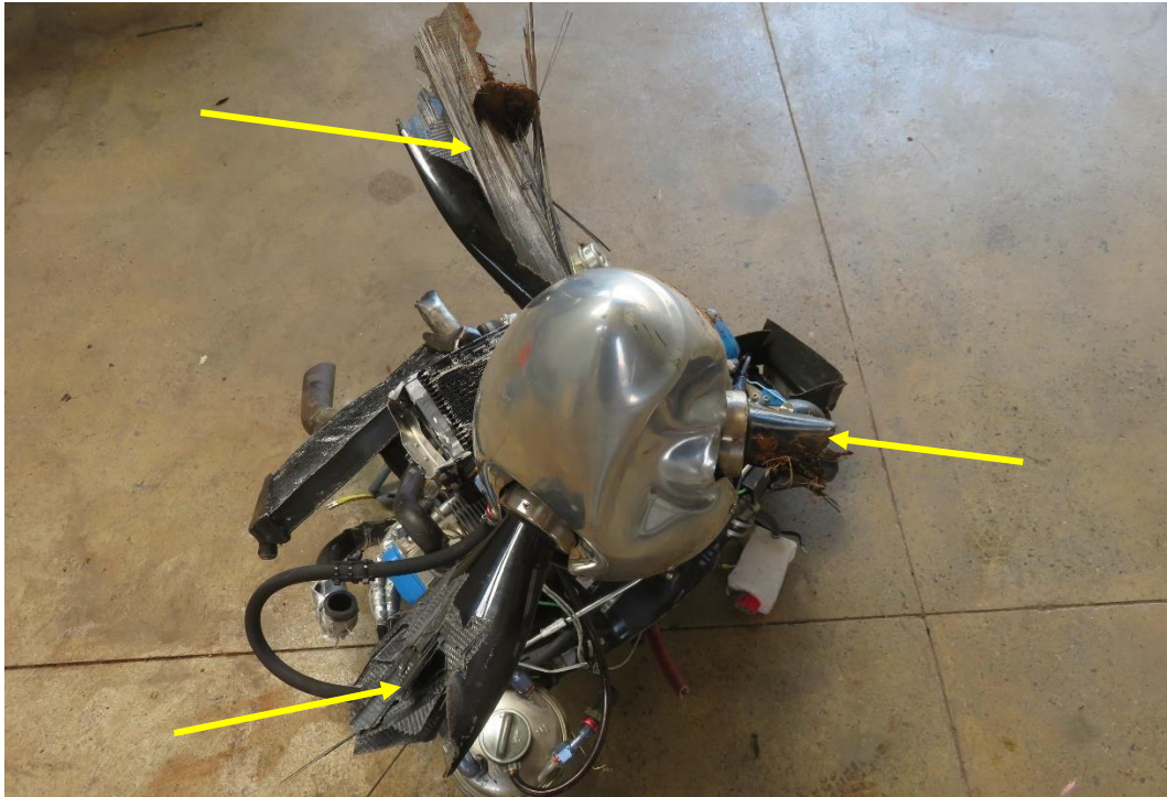
Figure 11: The view of the propeller with all three blades severed near the hub assembly.
