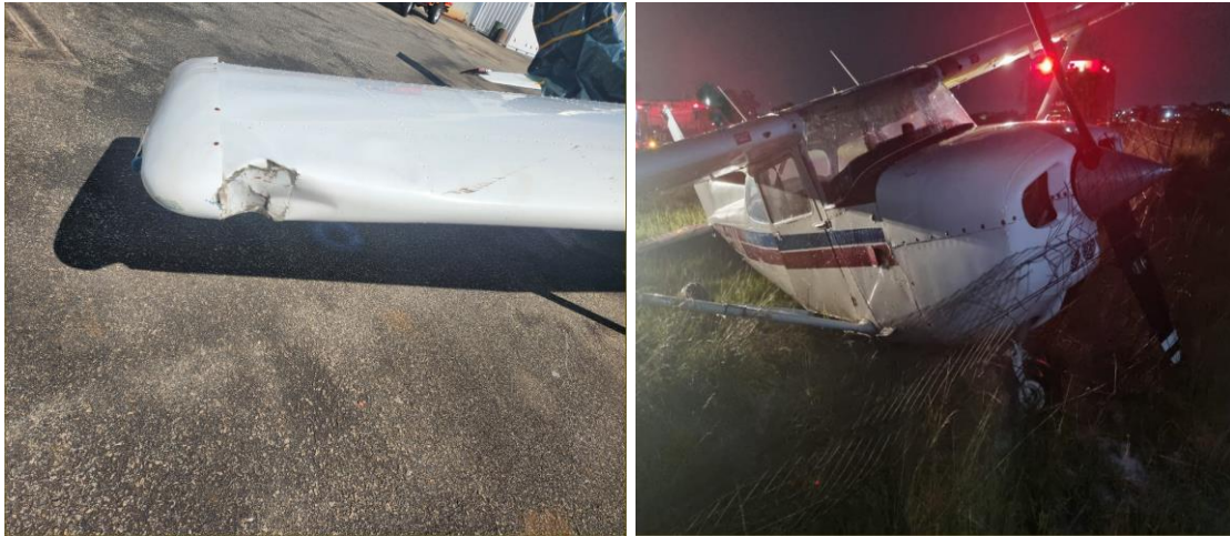
Figures 1 and 2: The damaged right-wing leading edge (right); and the aircraft against the perimeter fence. (Source: FAGC Fire Department)
