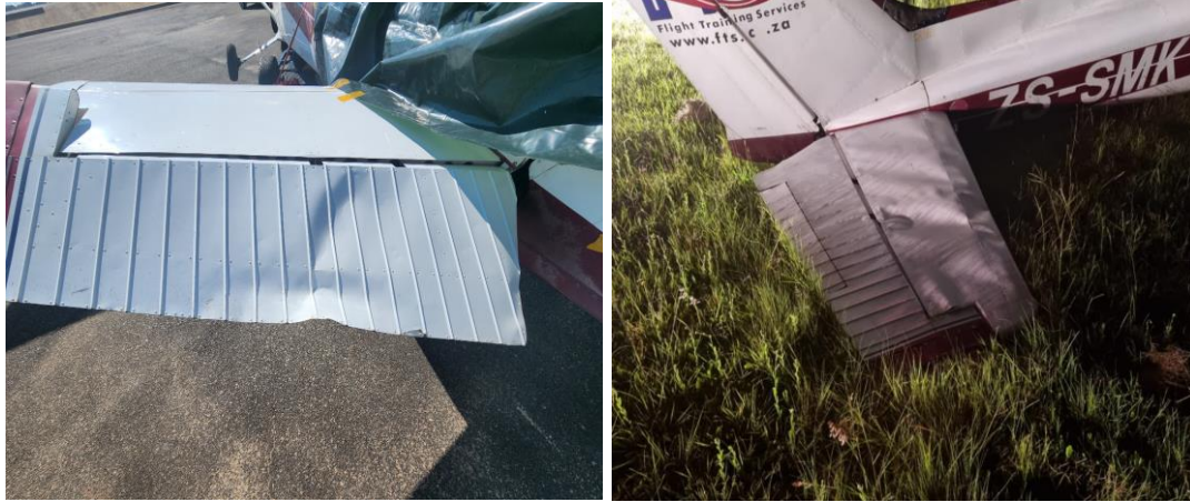
Figures 4 and 5: Damage to the left-side elevator and right-side horizontal stabiliser. (Source: FAGC Fire Department)
