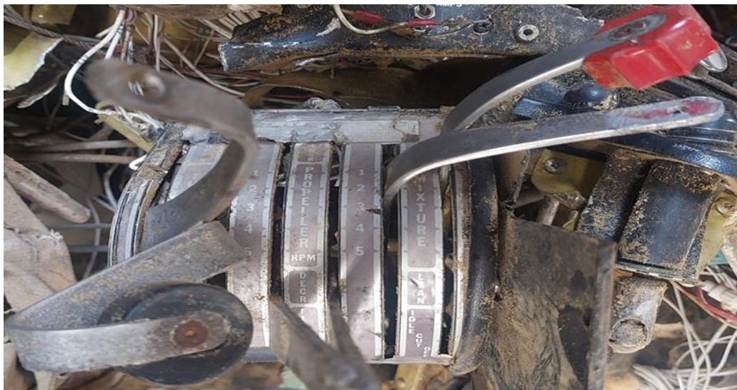
Figure 7: The console showing the position of the power levers.
