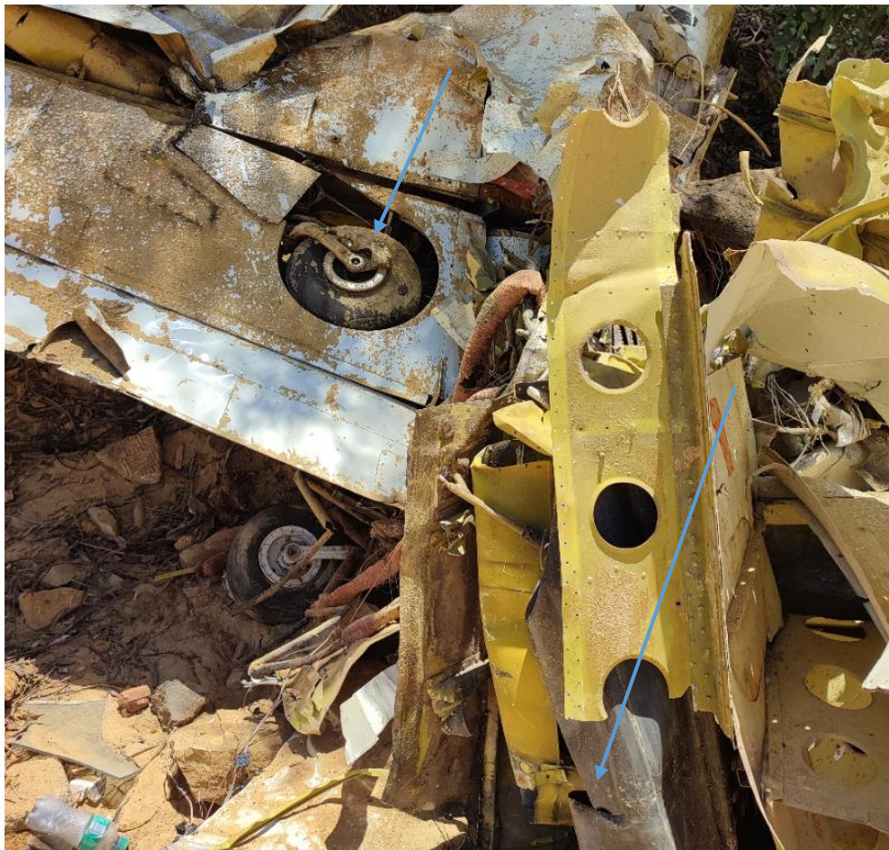
Figure 9: The ruptured fuel tank bladder and the right main gear in a retracted position.
