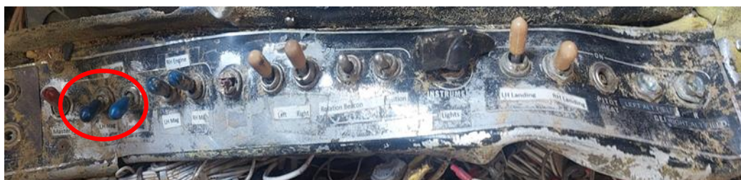
Figure 5: The cockpit instrument with the left-side magneto switch in the 'off' position.
