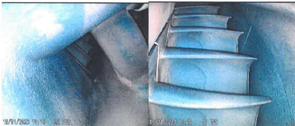
Figure 11: CT blades and the vane ring showing discolouration. (Source: AMO)
