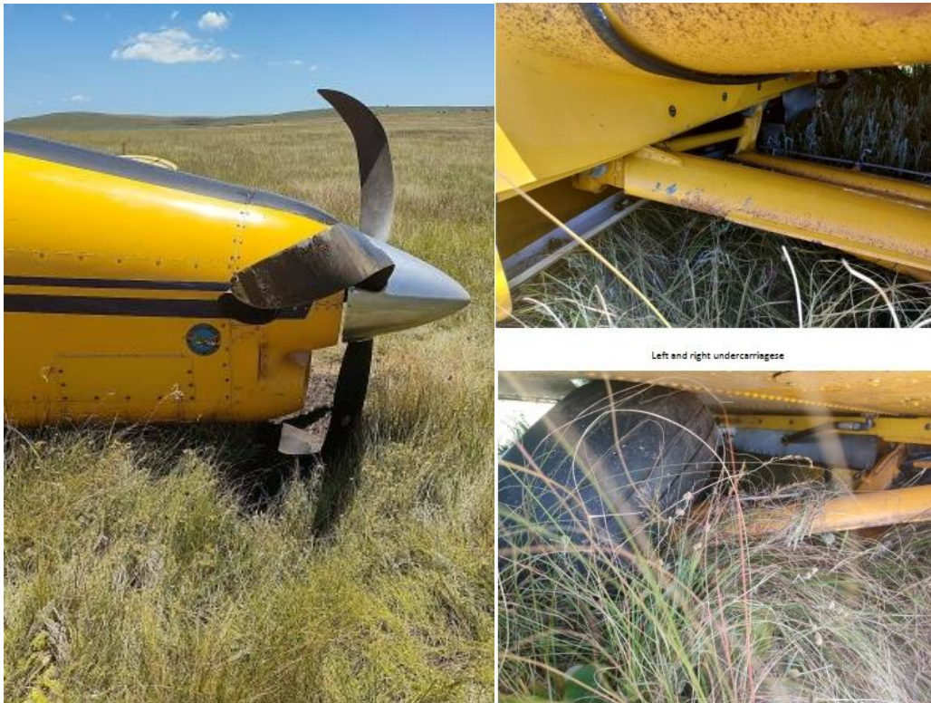
Figure 7: The damaged propeller (left) and main undercarriage (right). (Source: Operator)
