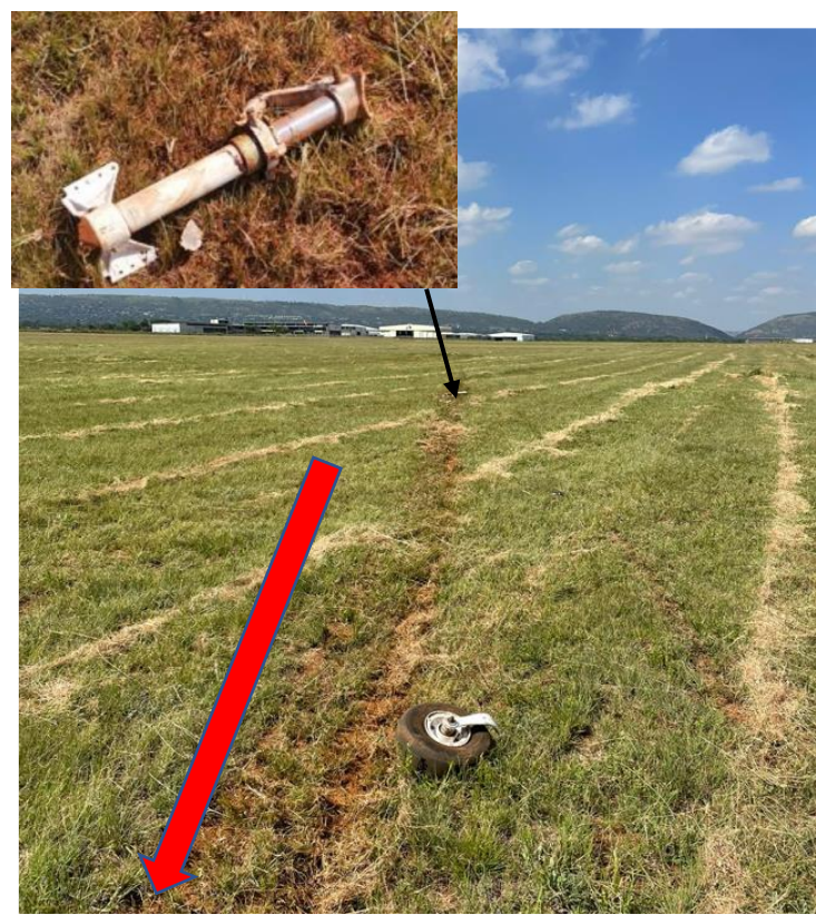
Figure 2: The nose strut and nose wheel after separating from the aircraft. The arrow shows the direction of the aircraft. (Source: Operator)
