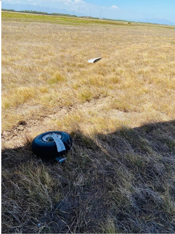
Figure 3: The detached nose wheel. (Source: Operator)
