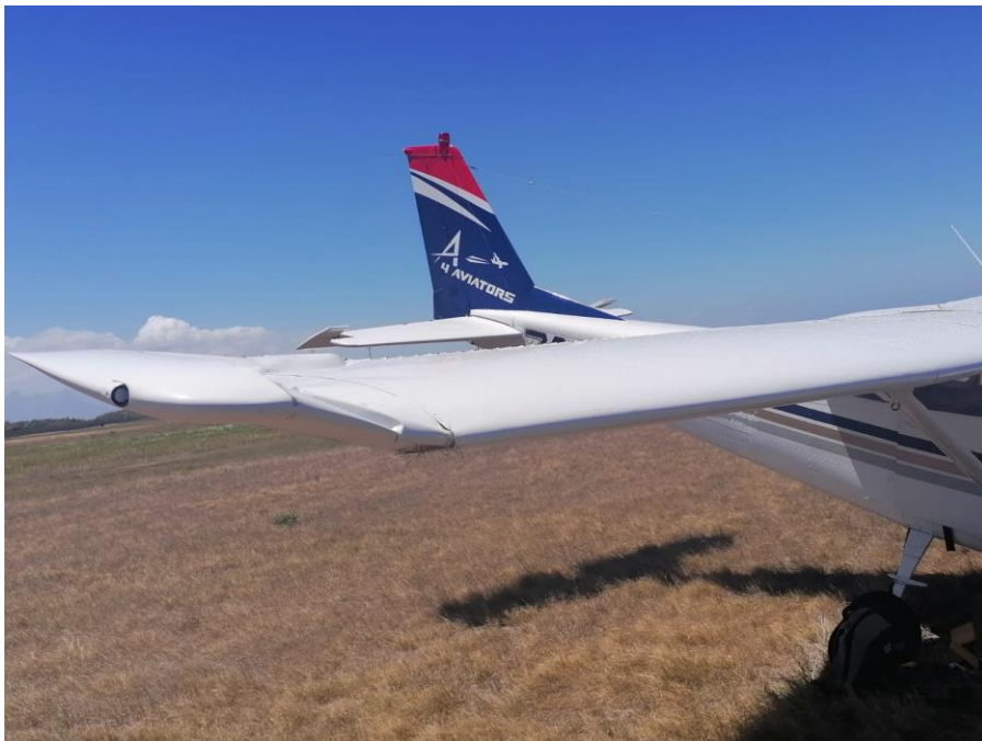
Figure 4: Damage on the right-wing tip. (Source: Operator)
