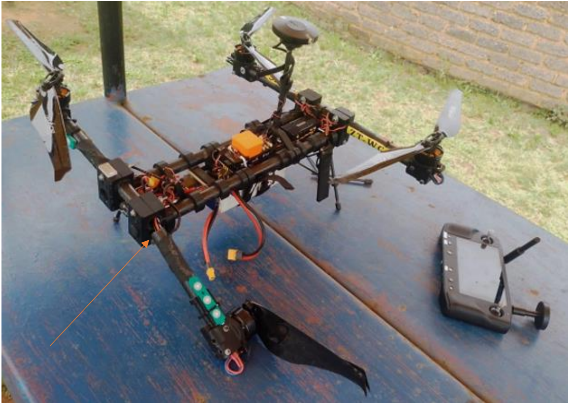
Figure 2: The damage on the right-side rear arm of the RPA.
