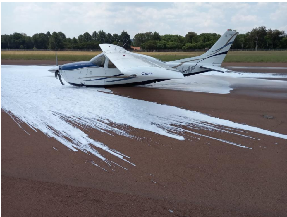
Figure 2: The chemical foam sprayed on the aircraft and the runway to prevent a possibility of fire eruption. (Source: Pilot)
