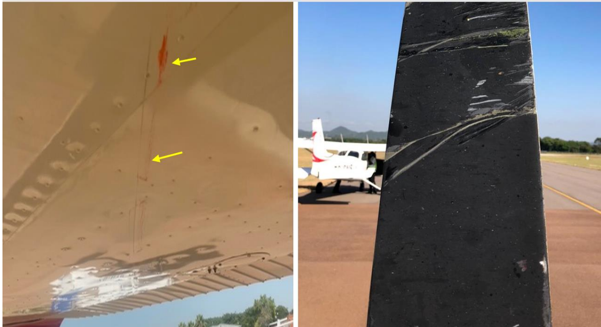
Figures 5 and 6: Scrape marks on the ZS-SCE aircraft right wing lower skin surface area and fairing (left picture). Witness marks on the blade as it cut through the ZS-SNS left wing tip (right picture).
