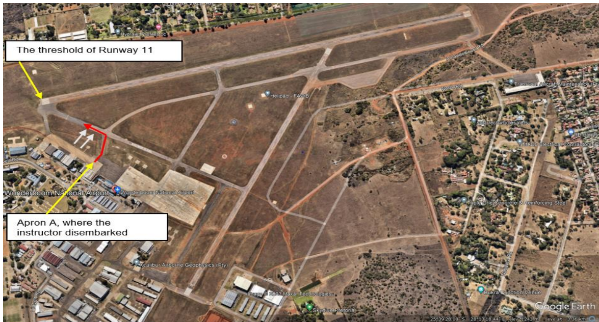
Figure 1: FAWB layout. The two white arrows indicate the position of the two stationary aircraft the ZS-SNS collided with on taxiway Delta to Runway 11. (Source: Google Earth).
