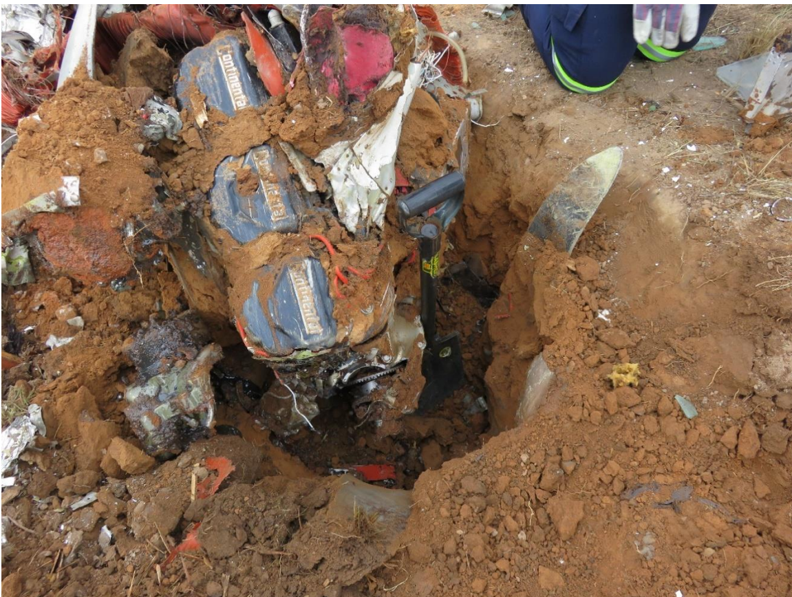
Figure 9: The engine after it was pulled out of the ground.
