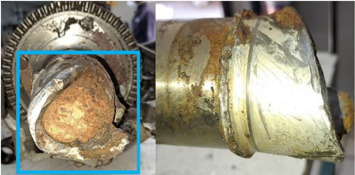
Figure 12: Enlarged view of the crankshaft driveshaft that failed under a torsion load depicted by the blue square. (Source: Impact Analysis Report: Engine & Propeller Assy., Beechcraft E33 Aircraft No ZS-IBX)
