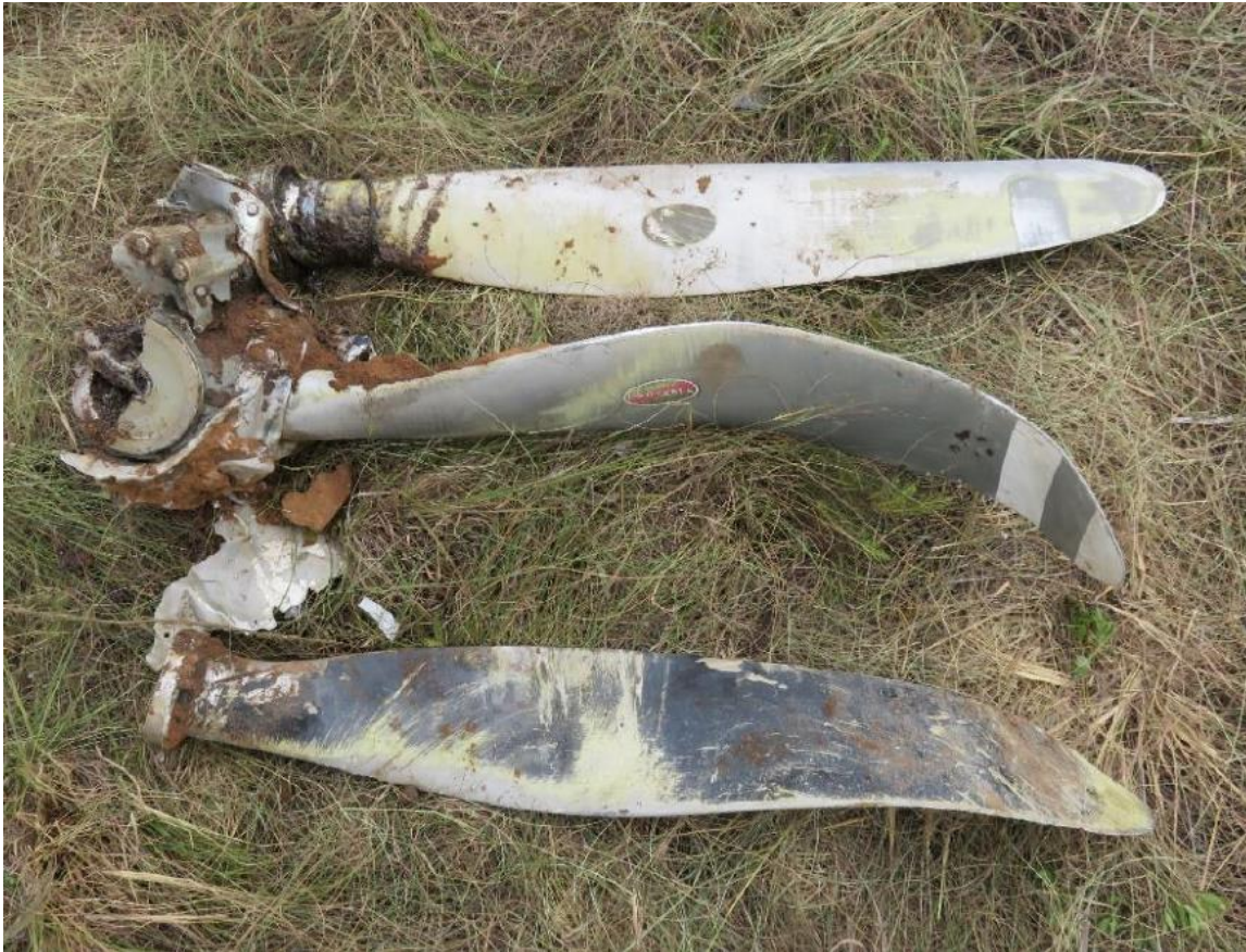
Figure 10: Damage to the propellor blades.
