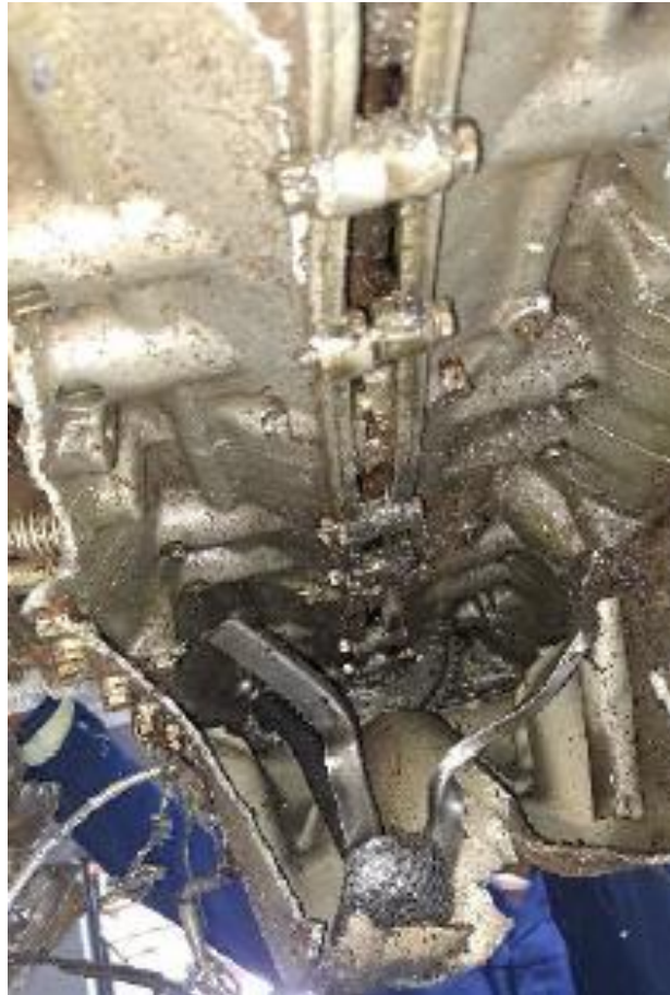
Figure 13: Crankcase showing several fractures and the oil sump section partially severed by the impact. (Source: Impact Analysis Report: Engine & Propeller Assy., Beechcraft E33 Aircraft No ZS-IBX)
