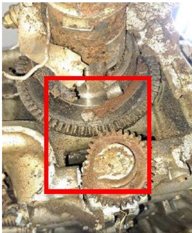
Figure 14: Damage to the governor drive bevel gear and pinion depicted by red square. (Source: Impact Analysis Report: Engine & Propeller Assy., Beechcraft E33 Aircraft No ZS-IBX)
