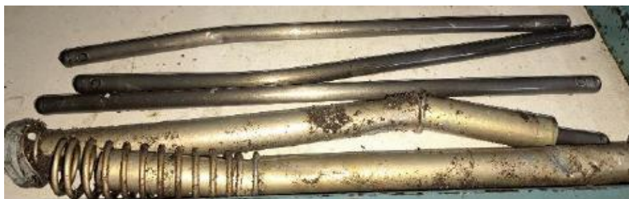
Figure 15: Pushrod housing and stems. (Source: Impact analysis report: engine & propeller assy., Beechcraft e33 aircraft No ZS-IBX)
