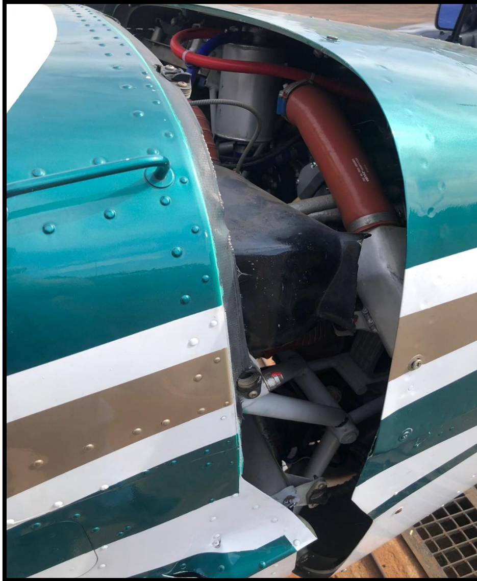
Figure 2: The firewall and airframe damage. (Source: Operator)
