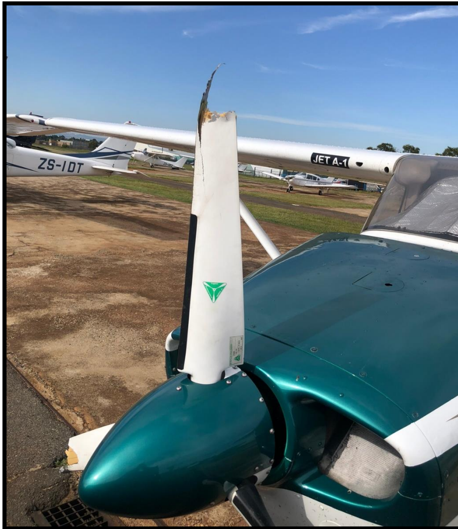
Figure 1: The damaged propeller blades. (Source: Operator)
