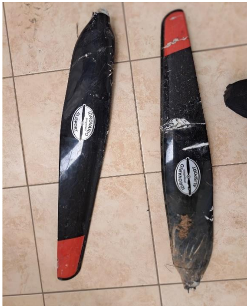
Figure 3: The damaged propellers.
