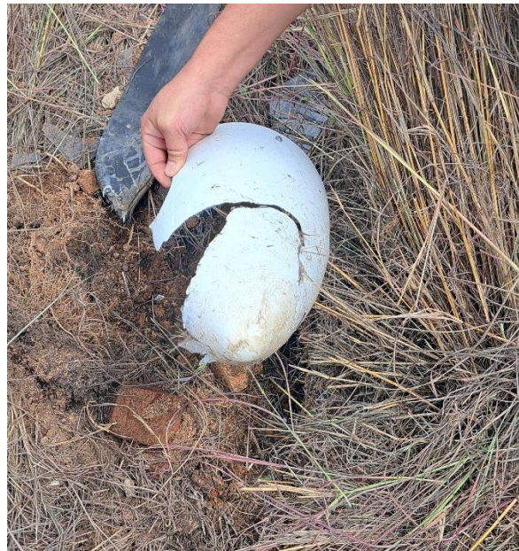
Figure 4: The cracked aircraft spinner.
