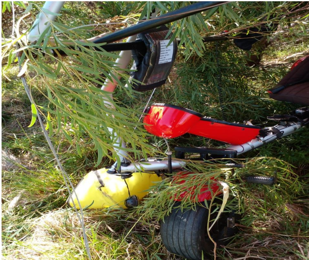
Figure 3: The damaged instrument pod and nose gear. (Source: Pilot)
