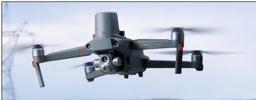
Figure 2: The DJI Mavic 2 Enterprise Advanced RPA type similar to the lost ZT-YIT. (Source: https://www.dji.com/mavic-2-enterprise-advanced )
