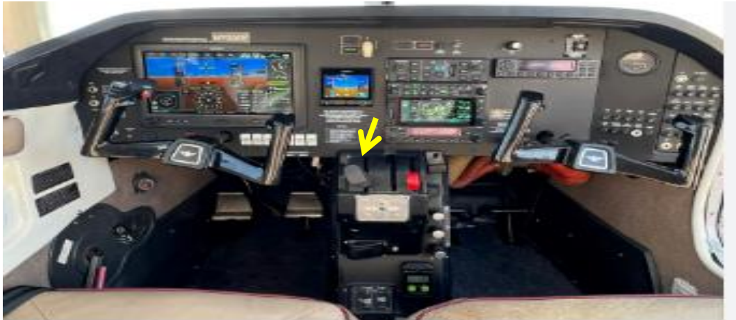
Figure 1: The instrument panel showing the landing gear control lever in the UP position. (Source: Operator)
