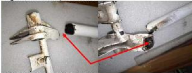
Photo 3: Fracture location (digital)
