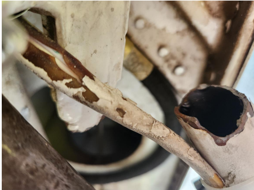
Figure 7: The failed bottom part of the drag brace.
