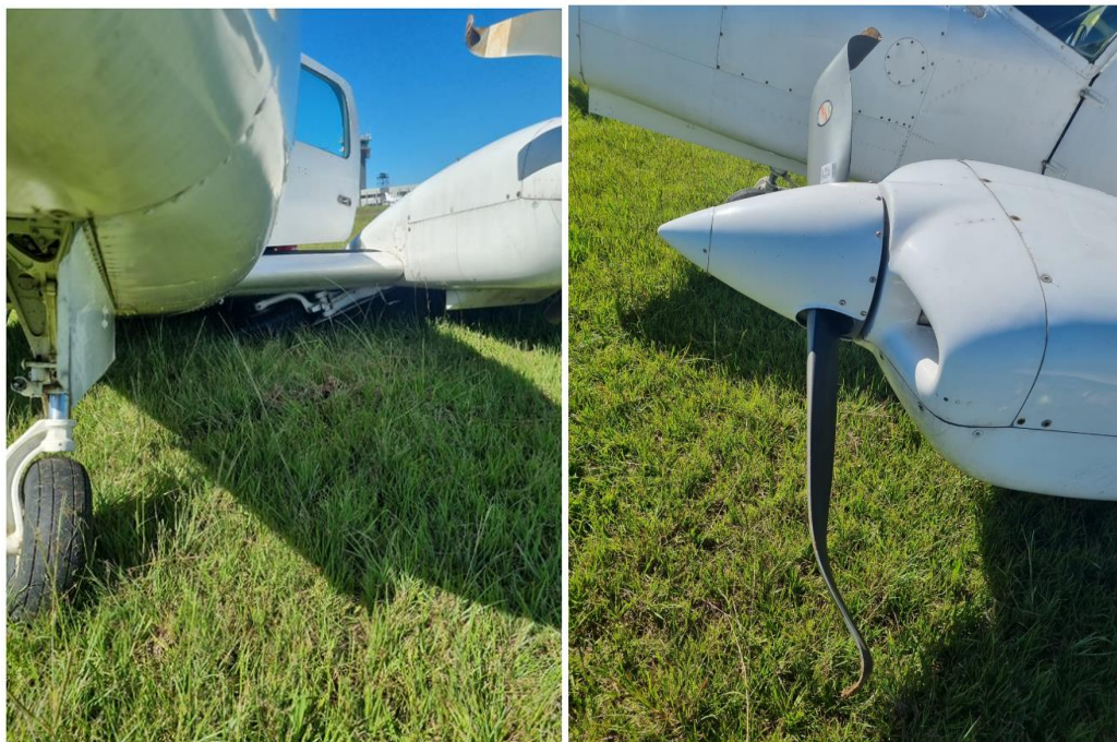
Figures 3 and 4: The collapsed landing gear (left) and the damaged propeller blades (right). (Source: FAGC Fire Department)
