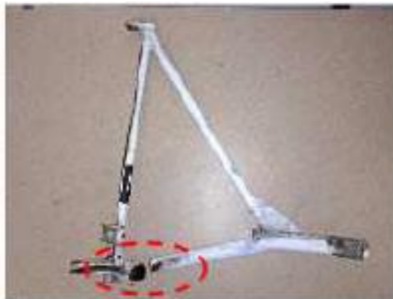
Photo 2: Main Landing Gear Leg, as supplied (digital)
