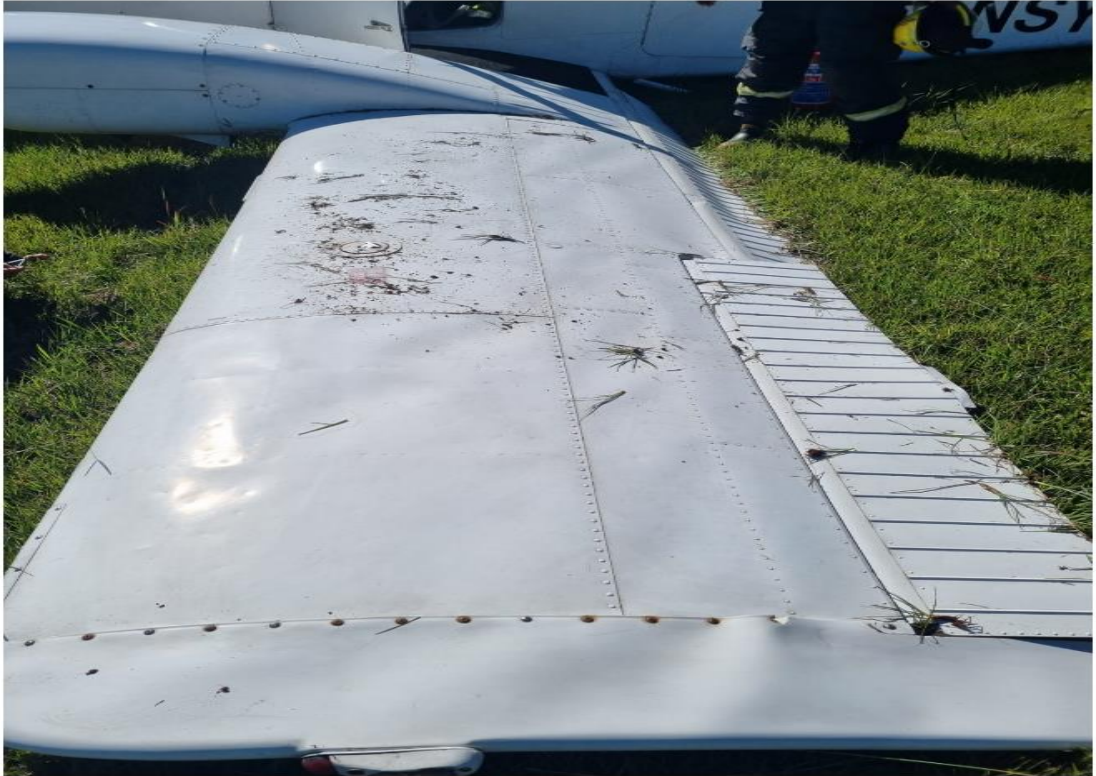
Figure 5: The damaged wing skin and the flight control surface. (Source: FAGC Fire Department)
