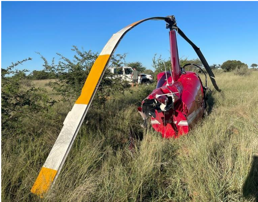
Figure 4: The aft view of the helicopter showing the severed tail boom. (Source: Pilot)
