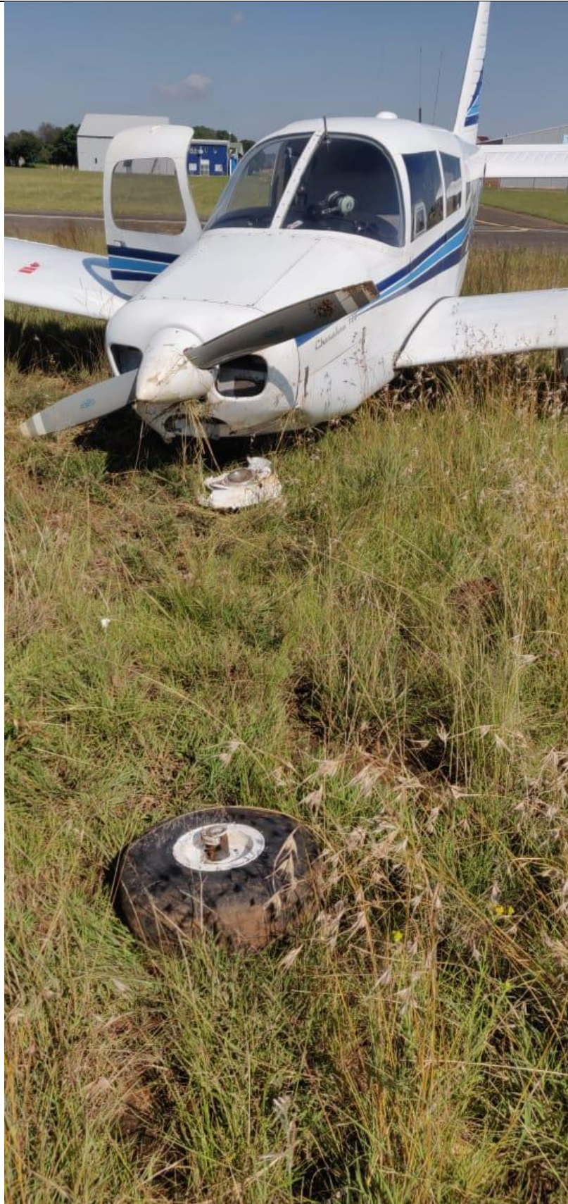
Figure 2: The front view of the aircraft and the nose wheel assembly that detached from the fork. (Source: Operator)
