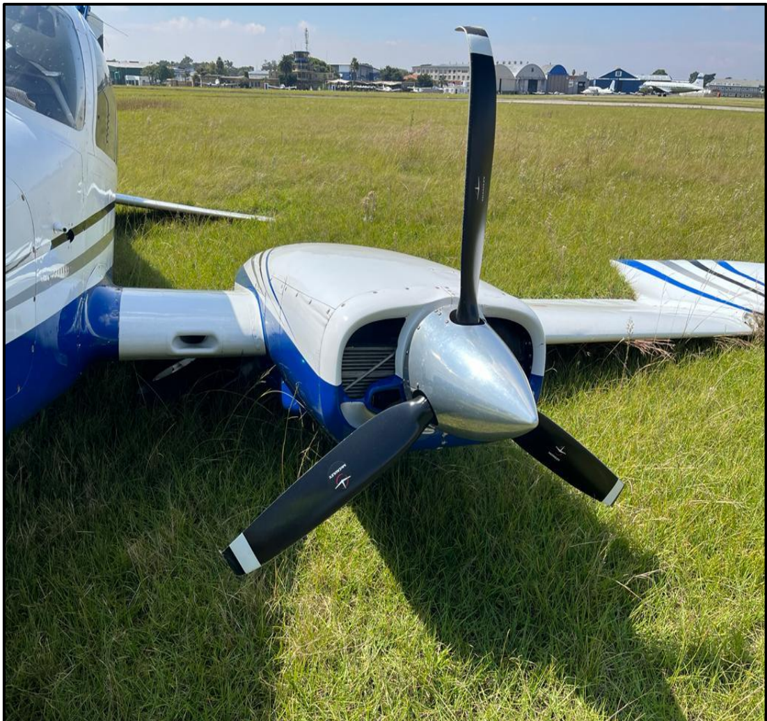
Figure 3: Damage sustained by the propeller.
