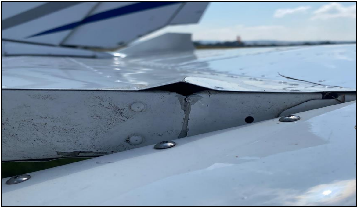
Figure 8: The damaged left elevator.
