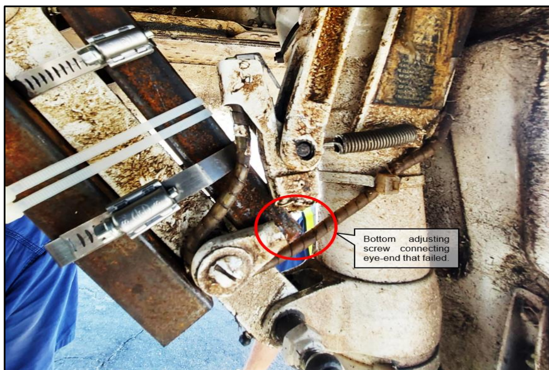
Figure 7: The left main landing gear supported with steel bars and the damaged bottom adjusting screw connecting eye-end.
