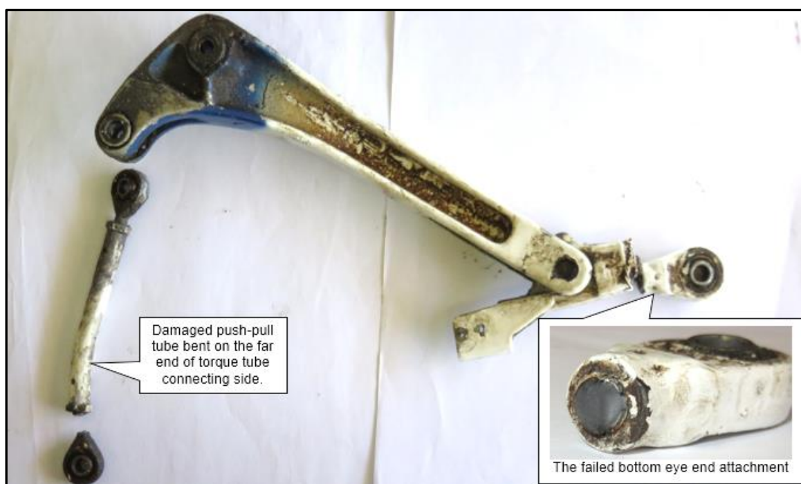
Figure 10: The damaged components.
