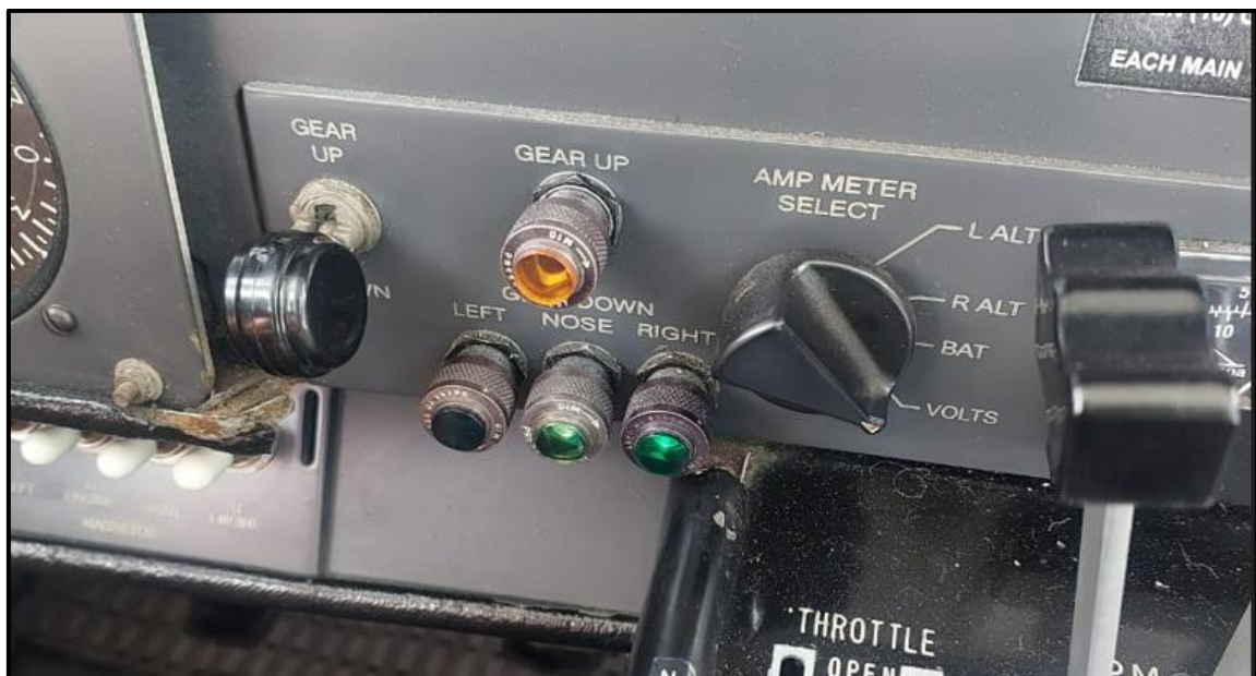
Figure 5: The cockpit landing gear controls and indicators.
