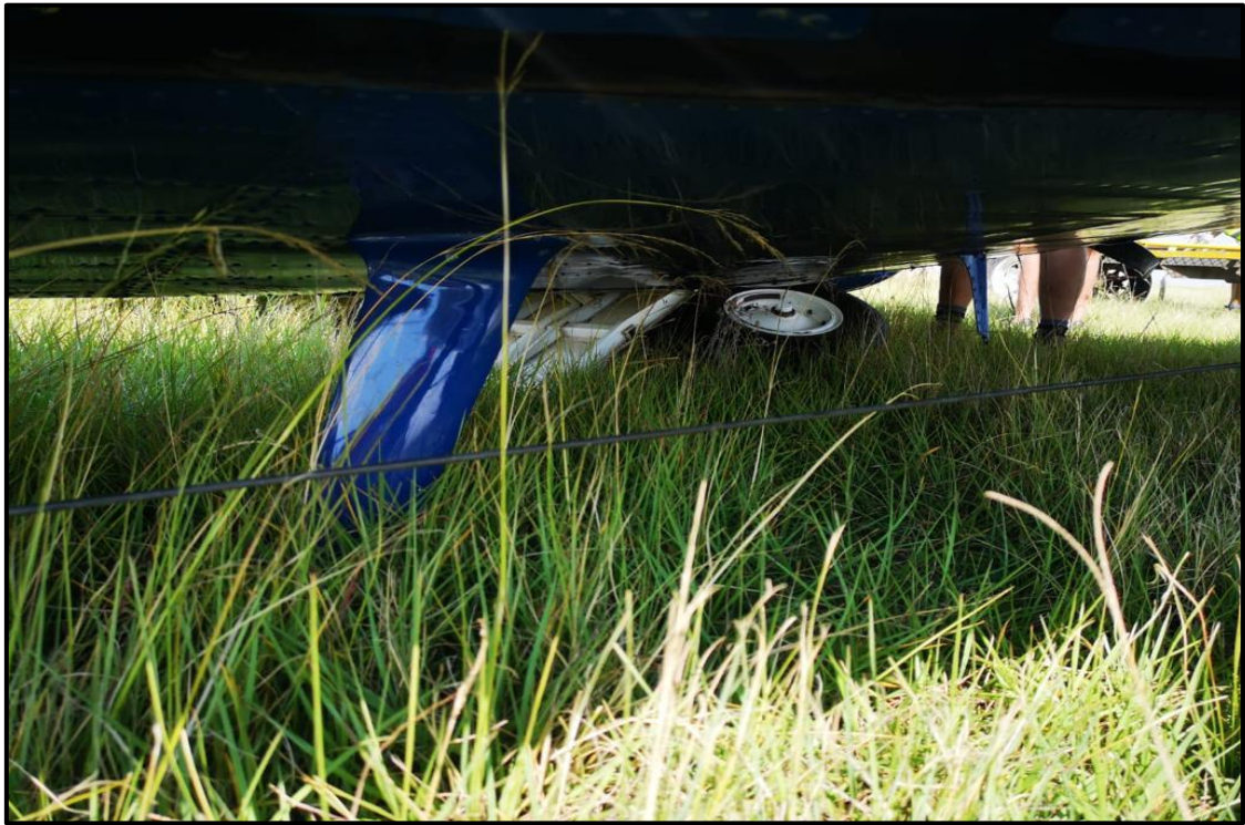
Figure 4: The collapsed left main landing gear.
