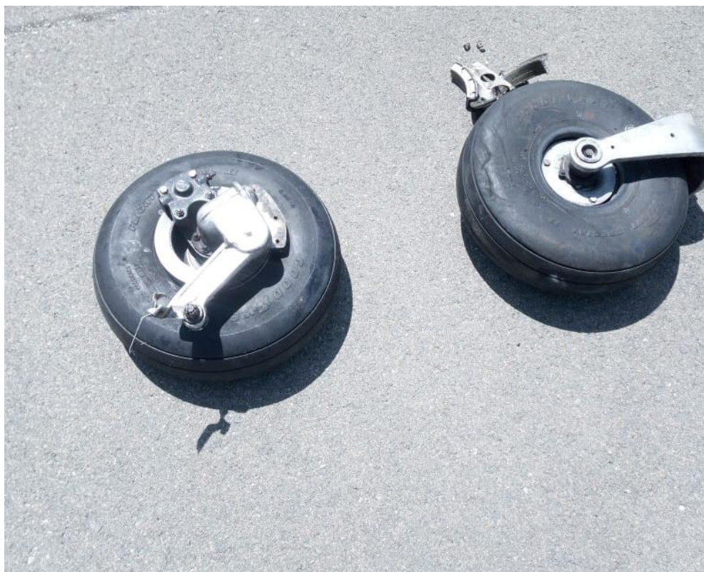
Figure 2: The nose and the right main wheels that separated during the accident. (Source: FALA Fire Department)
