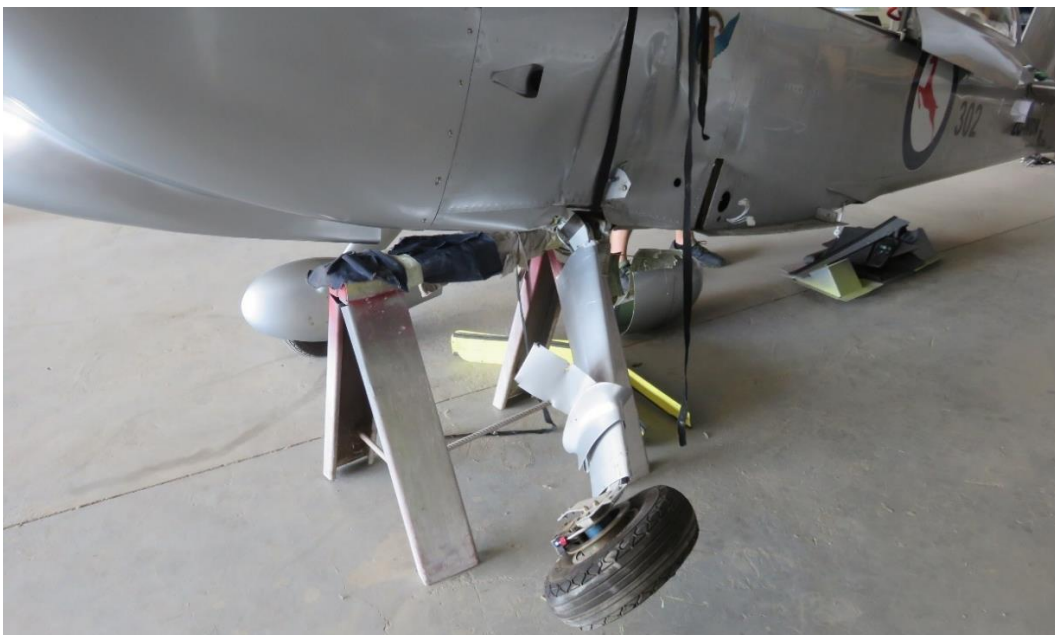
Figure 3: The damage caused to the left main gear.
