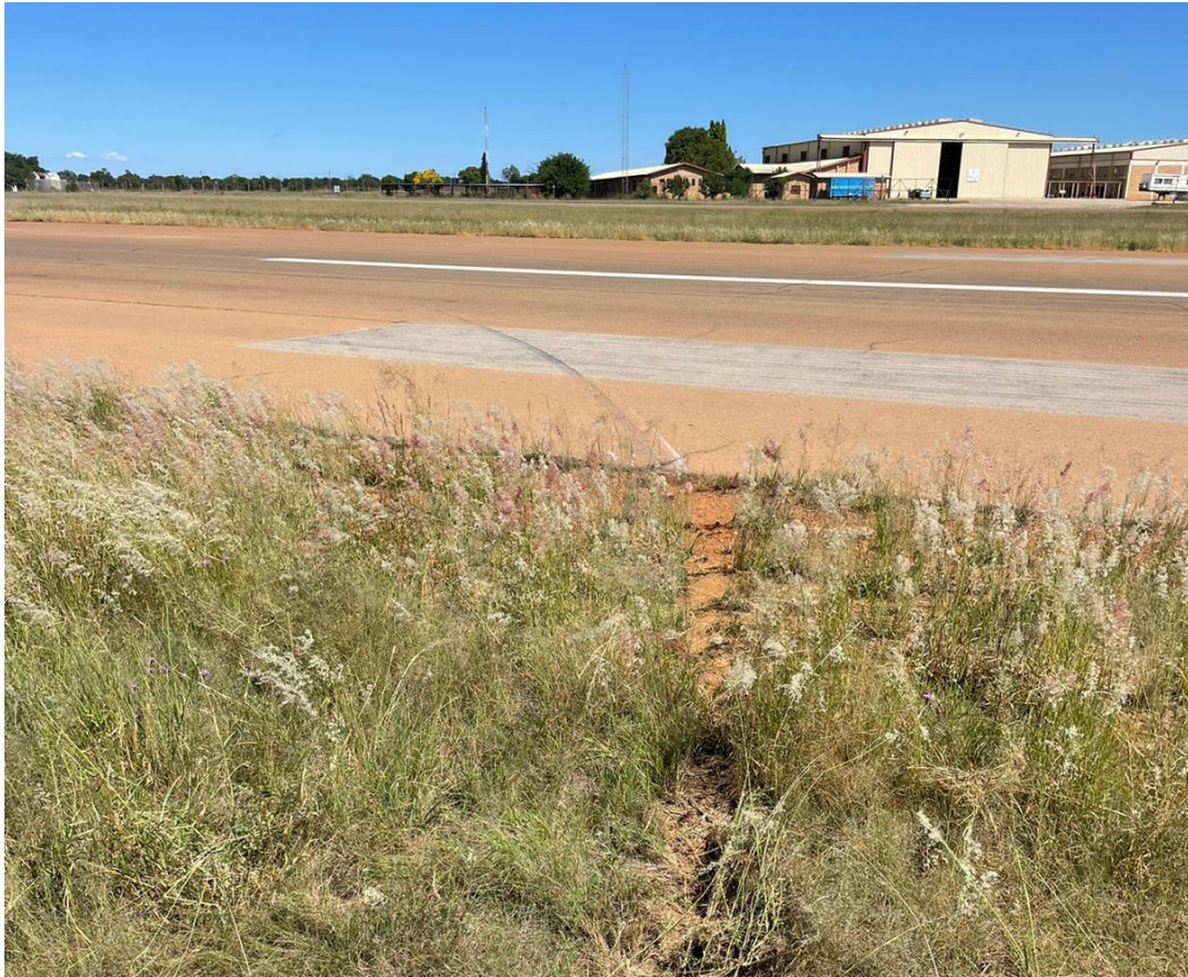
Figure 6: The left main tyre markings on the runway after the aircraft veered off.
