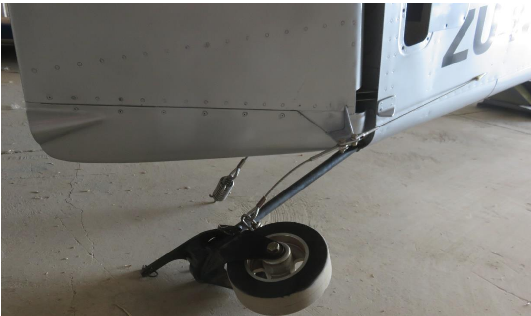
Figure 5: The tail wheel broke off during landing.
