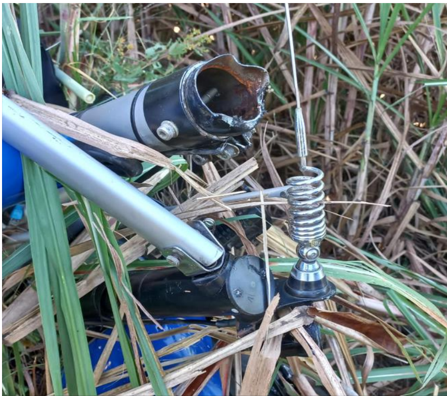
Figure 4: The broken bowsprit. (Source: Operator)
