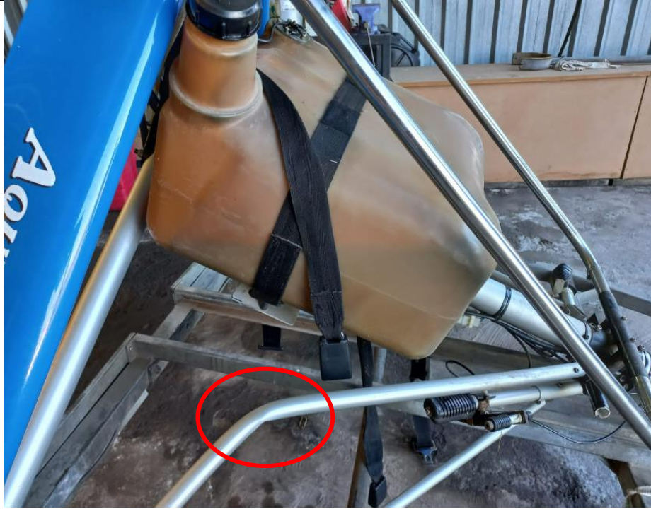
Figure 3: The bent right bowsprit. (Source: Operator)
