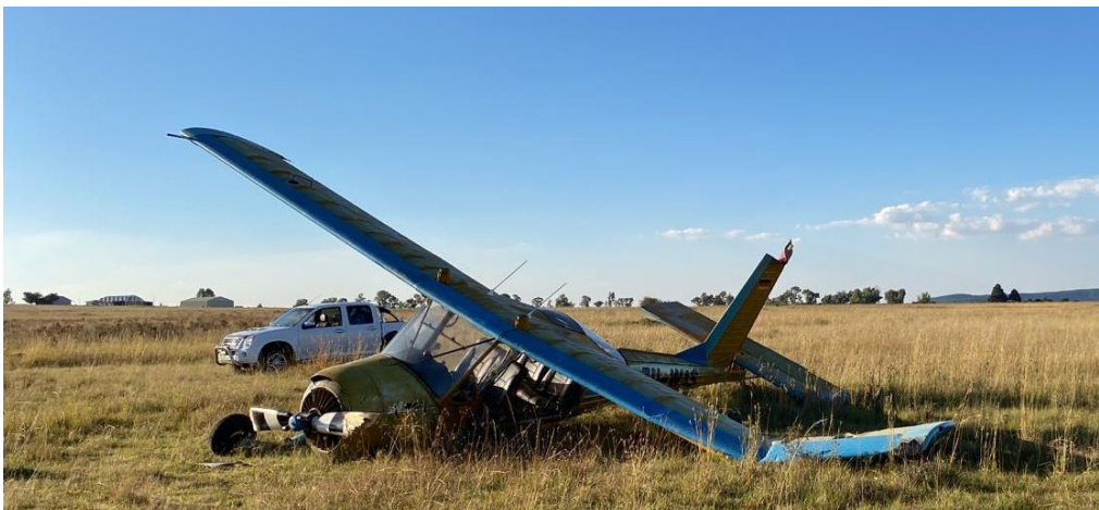
Figure 3: The left view showing the damaged wing. (Source: Operator)
