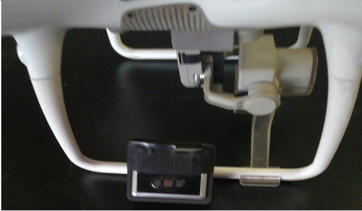
Figure 3: The new position of the Trackimo tracking module in a 3D printed holder attached to the skid. (Source: Operator)
