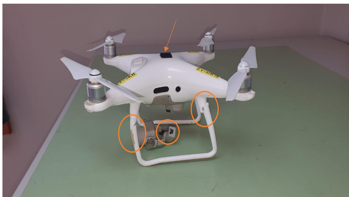
Figure 2: Damage to the aircraft (circled in orange). The orange arrow shows the Trackimo tracking module attachment point. (Source: Operator)
