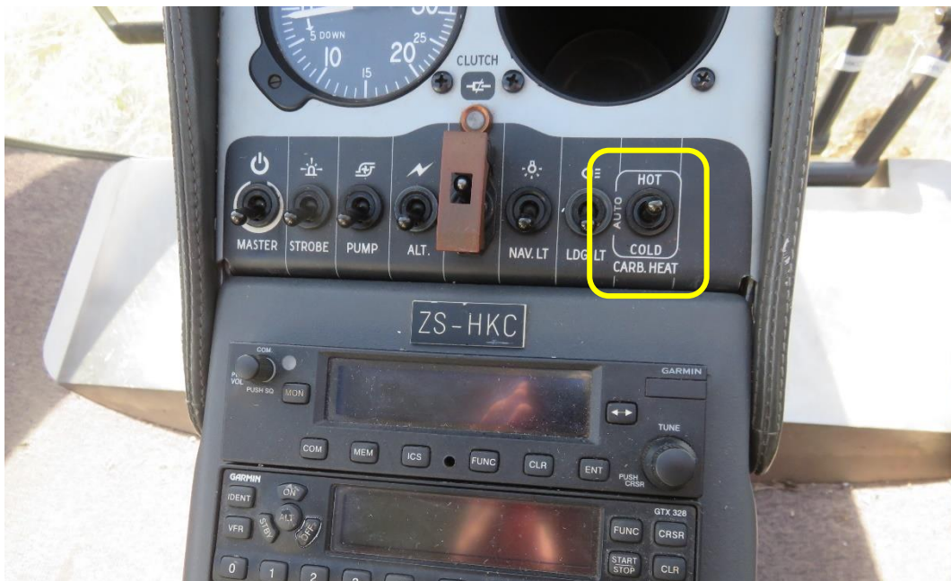
Figure 12: Instrument panel with the carb heat switch in the yellow window.
