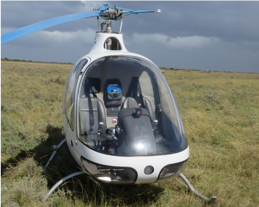
Figure 6: The front view of the helicopter with the blue blade severed near the hub assembly.
