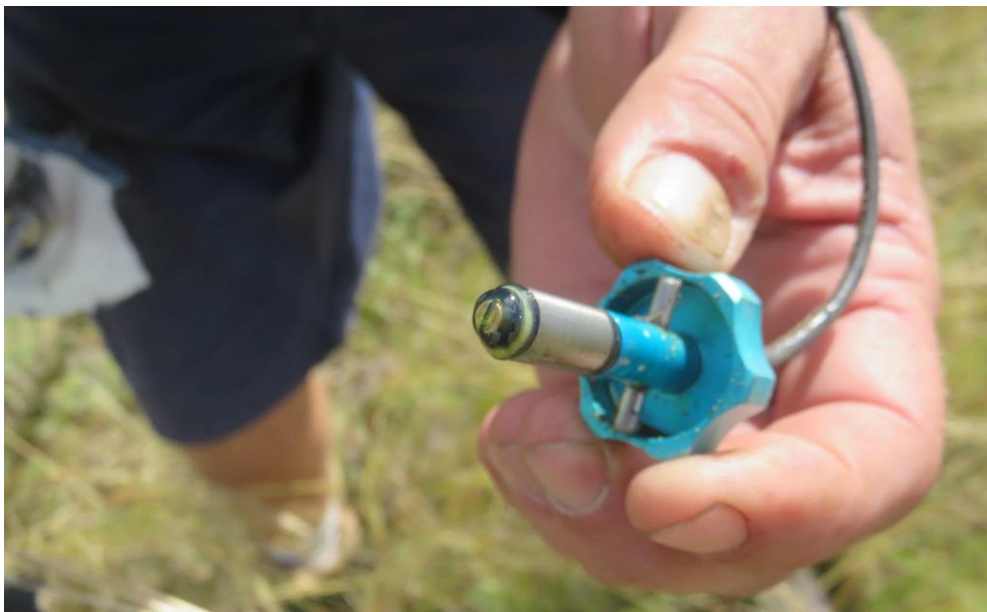
Figure 9: The magnetic chip detector on the tail rotor gearbox was clean.
