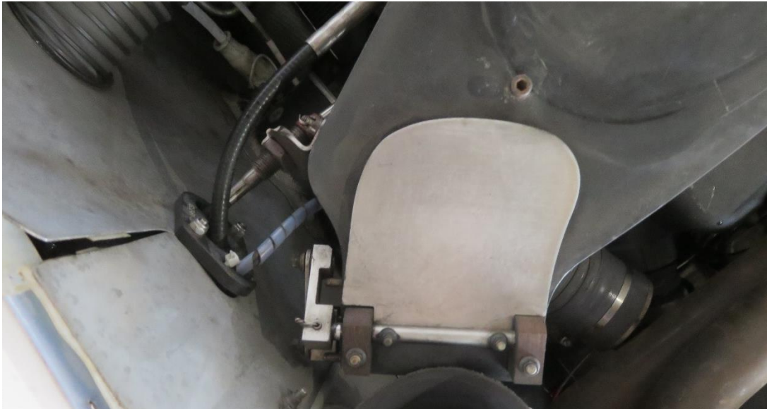
Figure 15: The valve in the close position.
