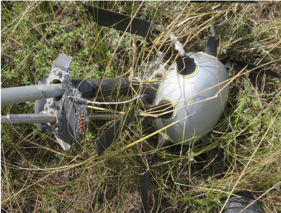
Figure 8: Substantially damaged fenestron and tail rotor drive shaft assembly.
