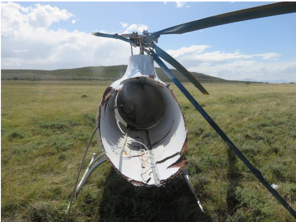
Figure 7: View of the aft position of the helicopter with the tail boom severed.
