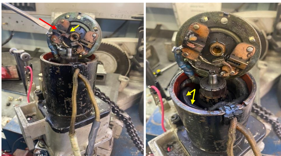
Figures 5 and 6: The landing gear power pack motor showing heat damage (left picture). Wetness on the wiring is caused by hydraulic fluid weep (right picture).
