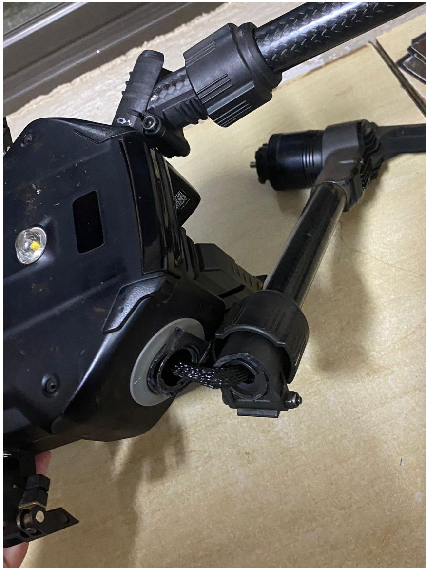
Figure 2: The damaged arm of the RPA.
