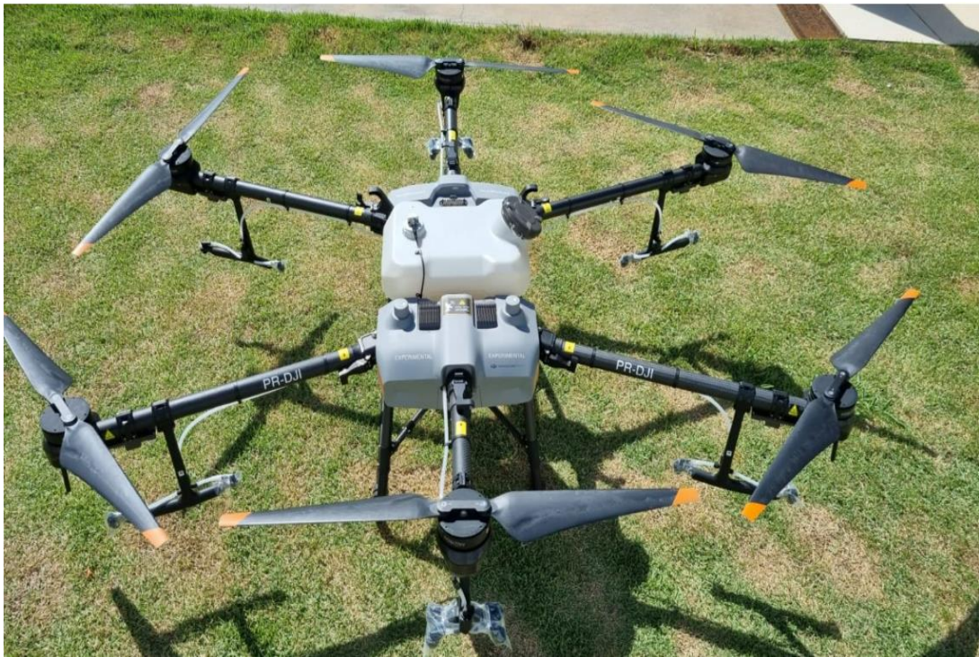
Figure 3: A picture of a DJI Agras T30 (New condition) similar to the accident RPA. (Source: Aldrones.com)
