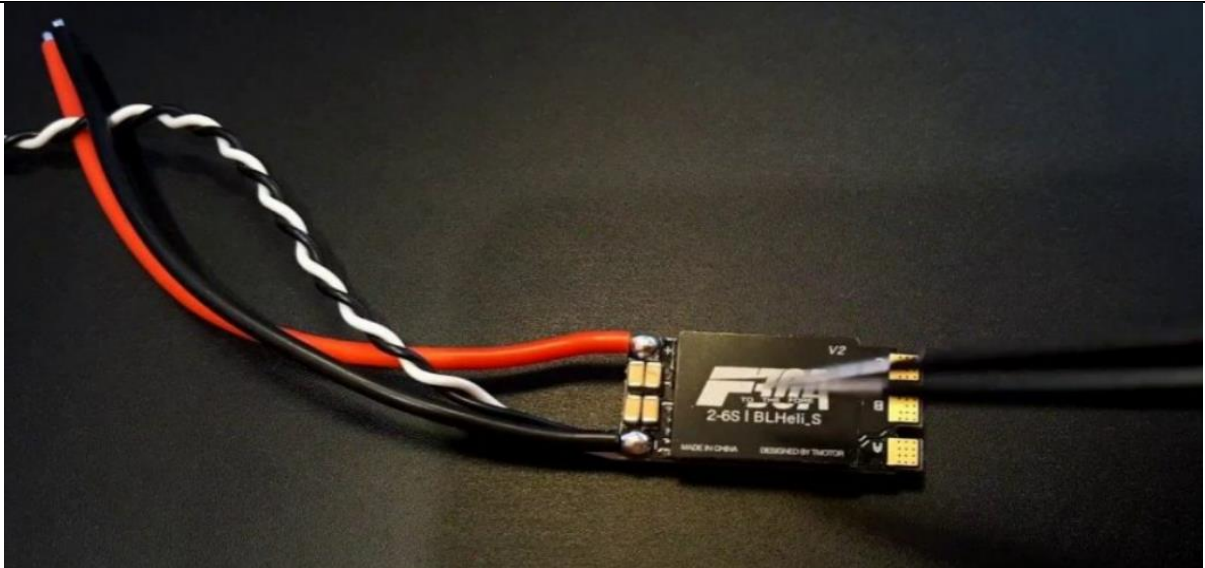
Figure 3: The electronic speed controller used on RPA.
